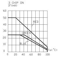
MAXIMUM FORWARD DC CURRENT VS, AMBIENT TEMPERATURE.
