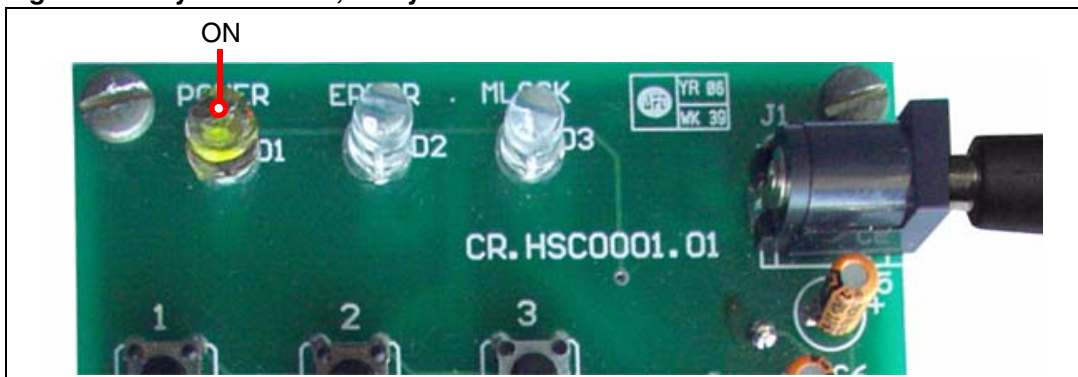
Figure 10. System stable, ready to use
