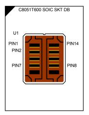
Figure 4. C8051T600 SOIC Socket Daughter Board (Included in Kit)
