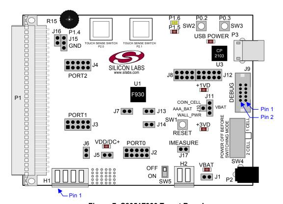
Figure 7. C8051F930 Target Board
