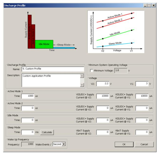
Figure 4. Battery Life Estimator Discharge Profile Editor
