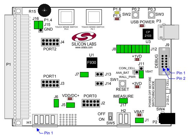
Figure 9. C8051F930 Target Board Shorting Blocks: Factory Defaults
