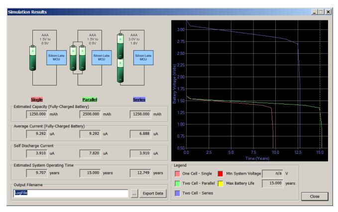
Figure 5. Battery Life Estimator Utility Simulation Results Form
