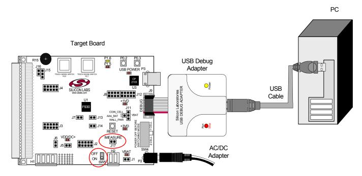
Figure 6. Hardware Setup using a USB Debug Adapter
