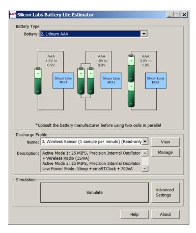
Figure 3. Battery Life Estimator Utility
