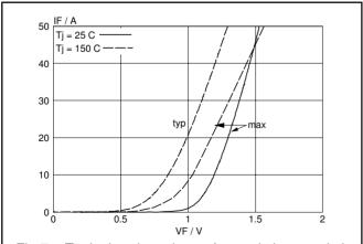
Fig.7. Typical and maximum forward characteristic  $I_F = f(V_F)$ ; parameter  $T_i$
