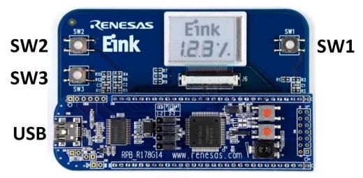
The kit comes pre-programmed with two demos. The kit requires power from a USB port and button S3 is used to switch between demos.
