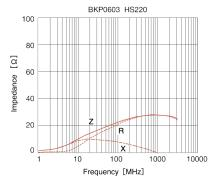
The data is reference only. Electrical characteristics vary depending on environment or measurement condition. TAIYO YUDEN reserves the right to make change to the Date at any time without notice. Before making final selection, please check product specification. 2013.10.29
