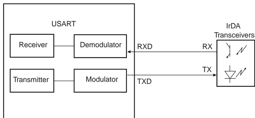
The receiver and the transmitter must be enabled or disabled according to the direction of the transmission to be managed.
