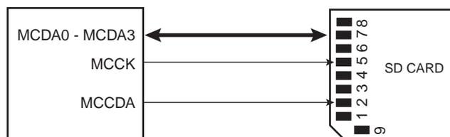
Note: When several HSMCI (x HSMCI) are embedded in a product, MCCK refers to HSMCI<sub>x</sub>\_CK, MCCDA to HSMCI<sub>x</sub>\_CDA, MCDA<sub>y</sub> to HSMCI<sub>x</sub>\_DAY.
