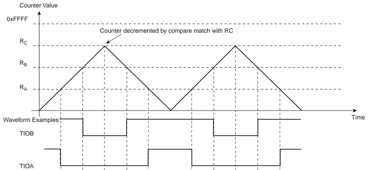
Figure 36-14. WAVSEL = 11 With Trigger
