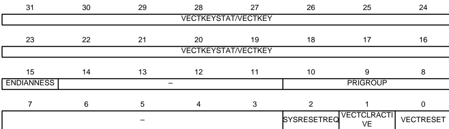
The SCB\_AIRCR register provides priority grouping control for the exception model, endian status for data accesses, and reset control of the system. To write to this register, write 0x5FA to the VECTKEY field, otherwise the processor ignores the write.
