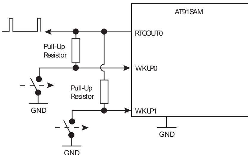
Figure 18-6. Low Power Debouncer (Push-to-Break switch, pull-down resistors)
