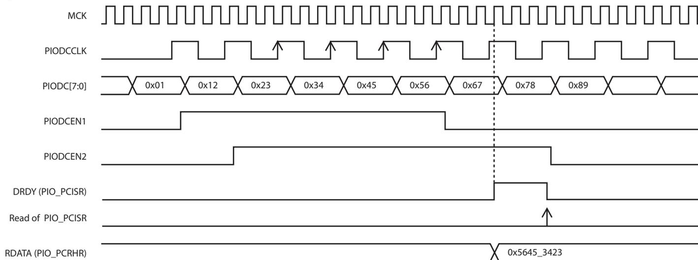
**Figure 30-11.Parallel Capture Mode Waveforms (DSIZE=2, ALWAYS=1, HALFS=0)**
