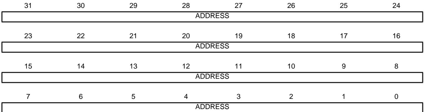
The MMFAR register contains the address of the location that generated a memory management fault.
