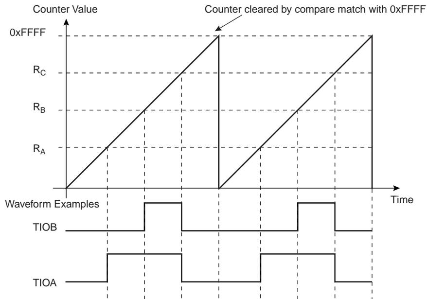
**Figure 36-8. WAVSEL= 00 with trigger**
