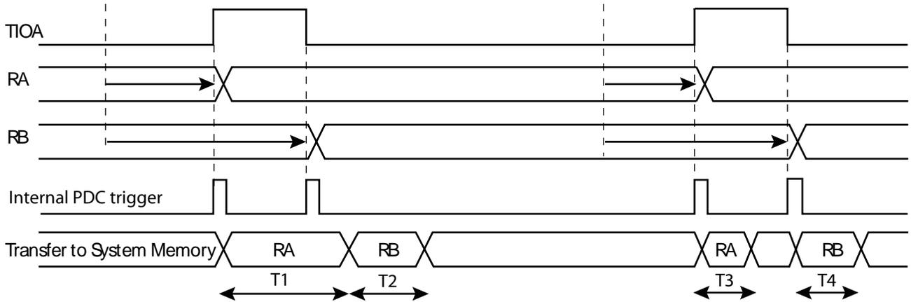
T1,T2,T3,T4 = System Bus load dependent ( $T_{min} = 8 \text{ MCK}$ )
