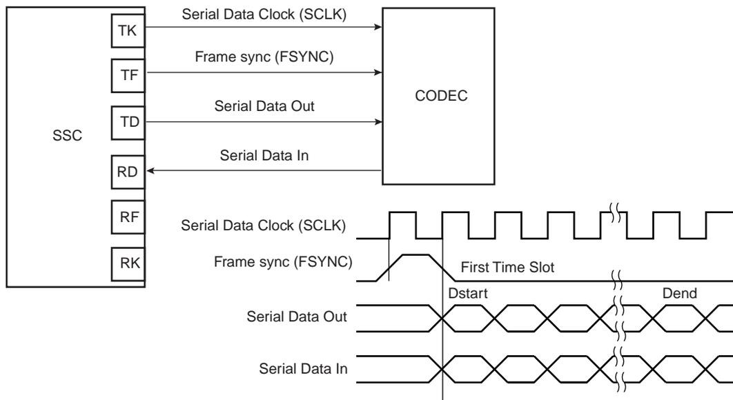
**Figure 31-19. Time Slot Application Block Diagram**
