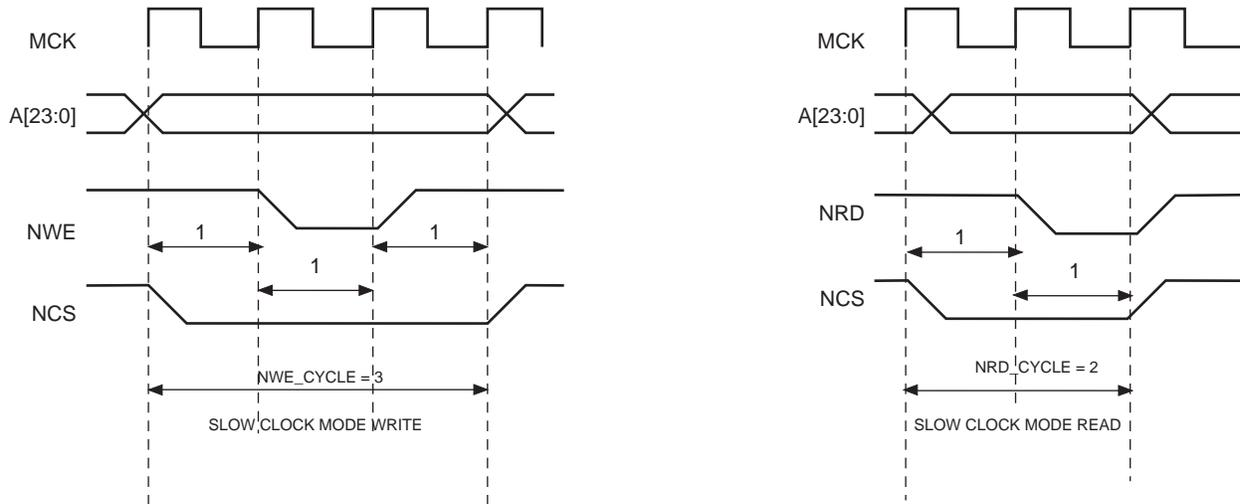
Table 26-4. Read and Write Timing Parameters in Slow Clock Mode
