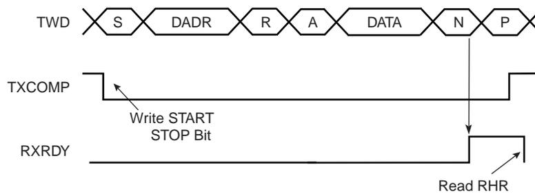
Figure 33-10. Master Read with Multiple Data Bytes
