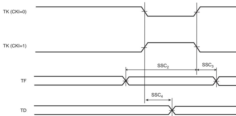
**Figure 43-21.SSC Transmitter, TK and TF as Input**
