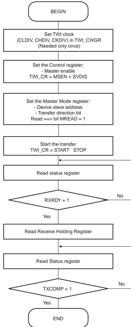
Figure 33-19. TWI Read Operation with Single Data Byte and Internal Address
