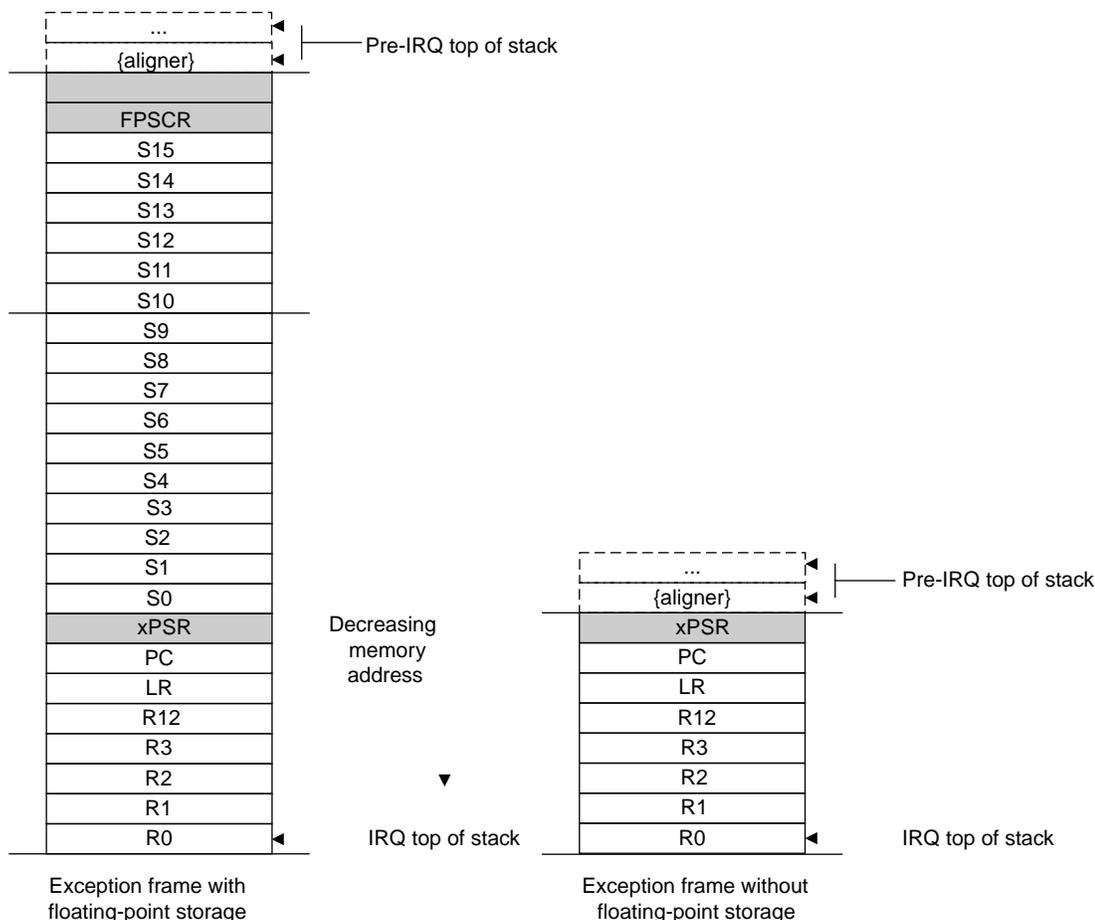
Immediately after stacking, the stack pointer indicates the lowest address in the stack frame. The alignment of the stack frame is controlled via the STKALIGN bit of the Configuration Control Register (CCR).
