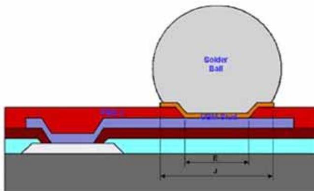
**Table 44-20. WLCSP Package Reference - Soldering Information (Substrate Level)**
