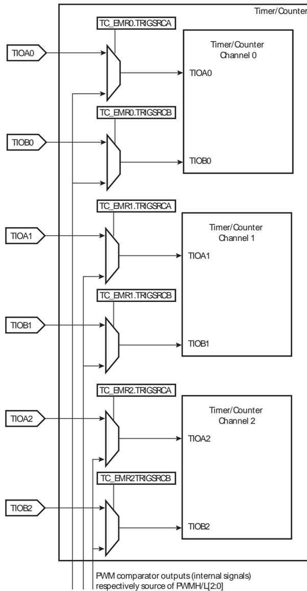
The output controller defines the output level changes on TIOA and TIOB following an event. TIOB control is used only if TIOB is defined as output (not as an external event).
