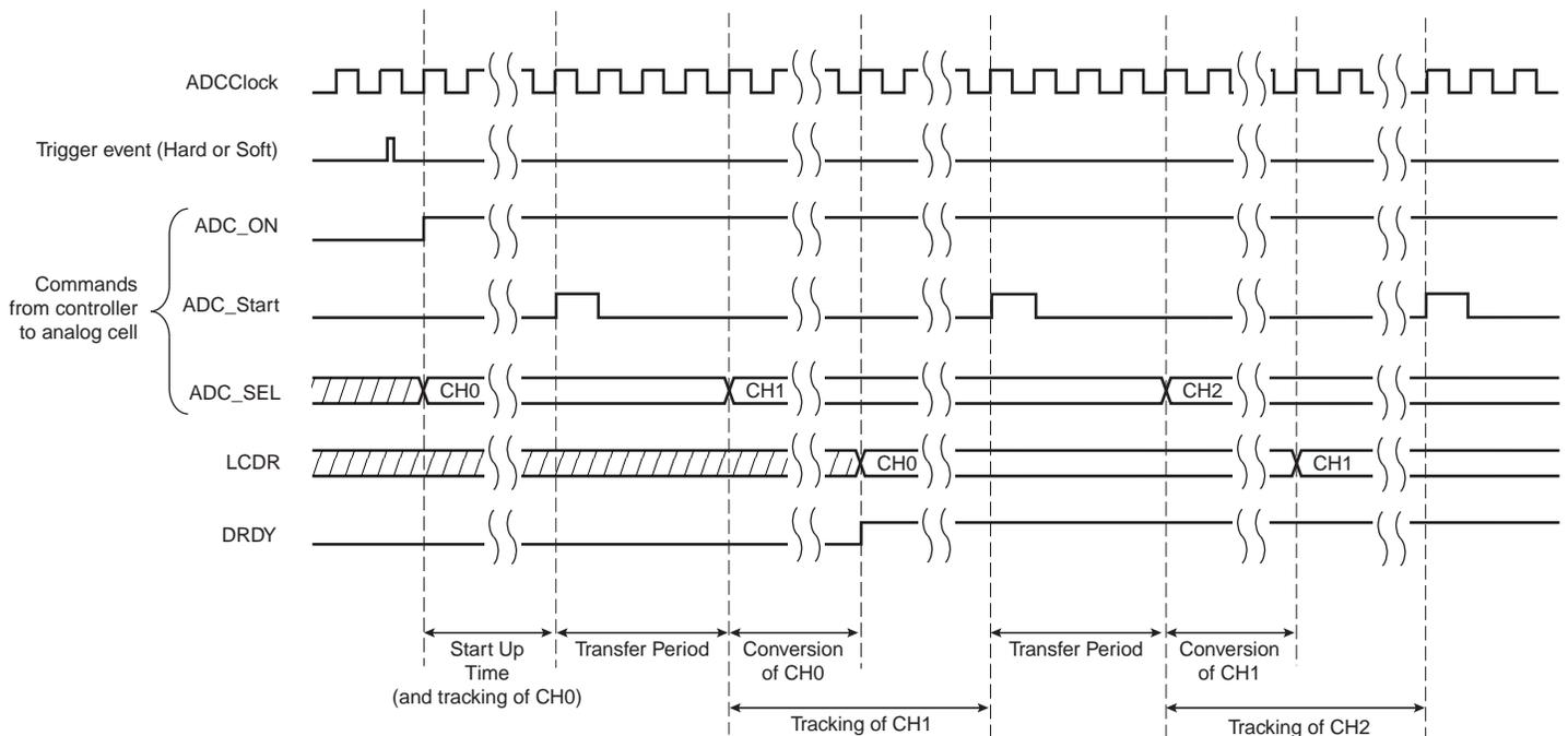
**Figure 41-3. Sequence of ADC conversions when Tracking time < Conversion time**
