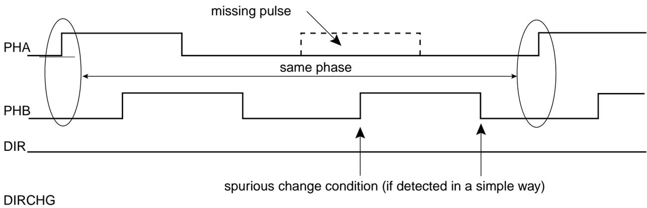
The direction change detection is disabled when QDTRANS is set to 1 in TC\_BMR. In this case the DIR flag report must not be used.
