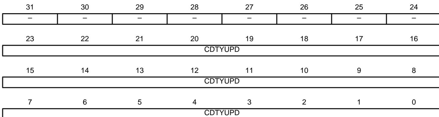
This register acts as a double buffer for the CDTY value. This prevents an unexpected waveform when modifying the waveform duty-cycle.
