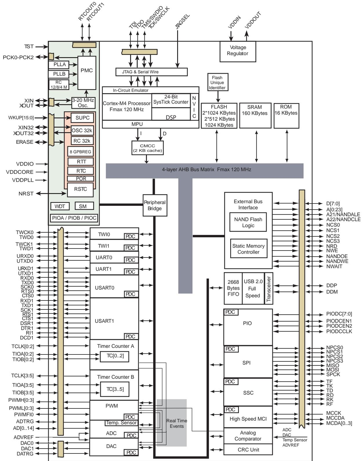
Figure 2-4. SAM4SD32/SD16/SA16 64-pin version Block Diagram
