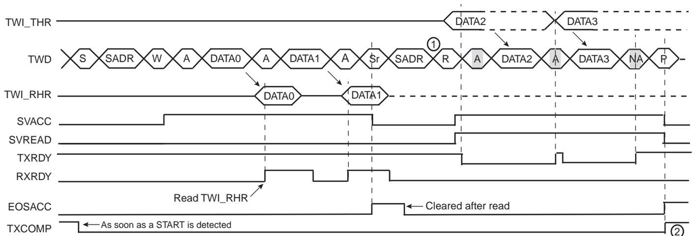
Notes: 1. In this case, if TWI\_THR has not been written at the end of the read command, the clock is automatically stretched before the ACK.
