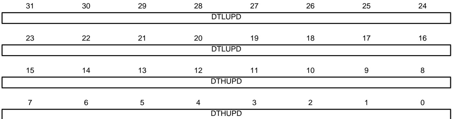
This register can only be written if the bits WPSWS4 and WPHWS4 are cleared in “PWM Write Protect Status Register” on page 913.
