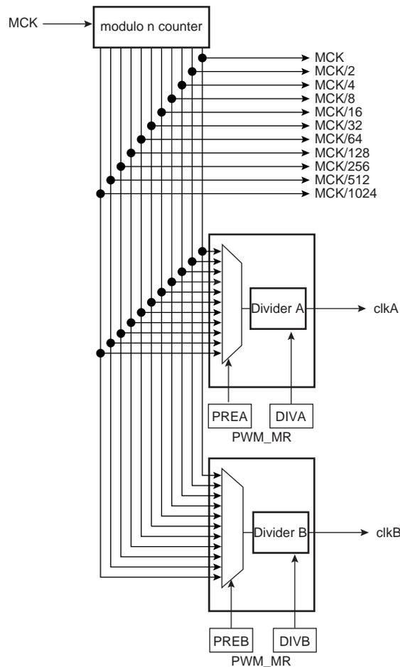
The PWM master clock (MCK) is divided in the clock generator module to provide different clocks available for all channels. Each channel can independently select one of the divided clocks.
