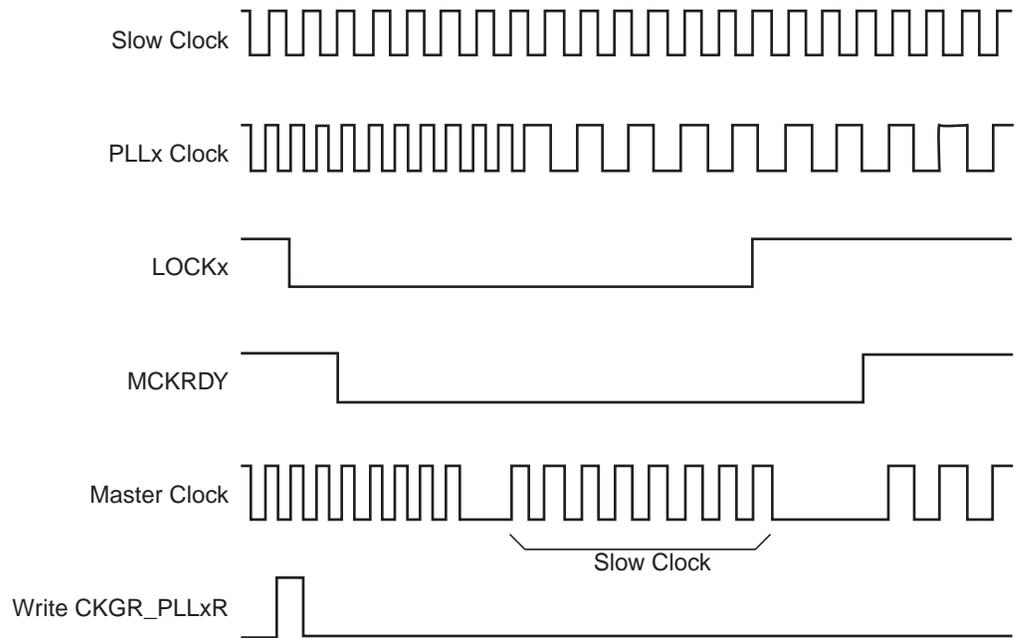
**Figure 28-12. Programmable Clock Output Programming**
