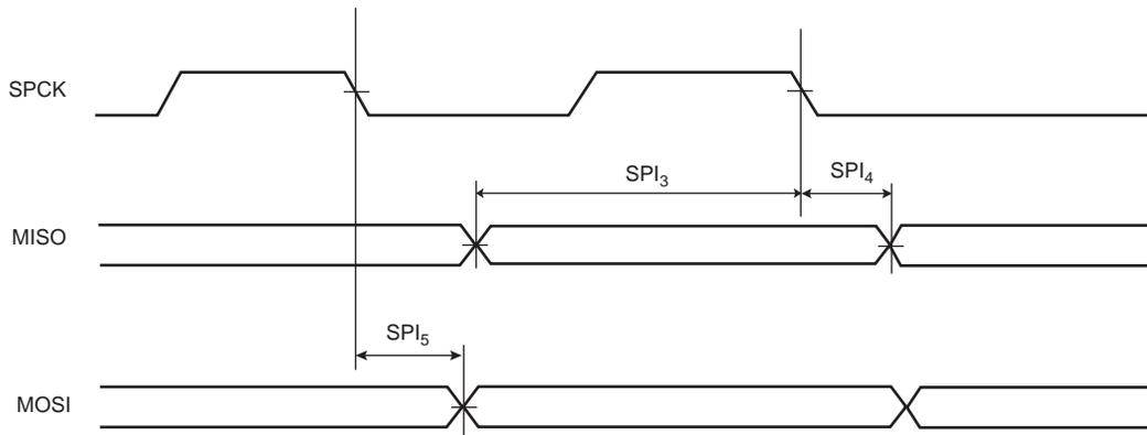
**Figure 43-16. SPI Slave Mode with (CPOL= 0 and NCPHA = 1) or (CPOL = 1 and NCPHA = 0)**
