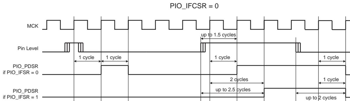
**Figure 30-6. Input Debouncing Filter Timing**
