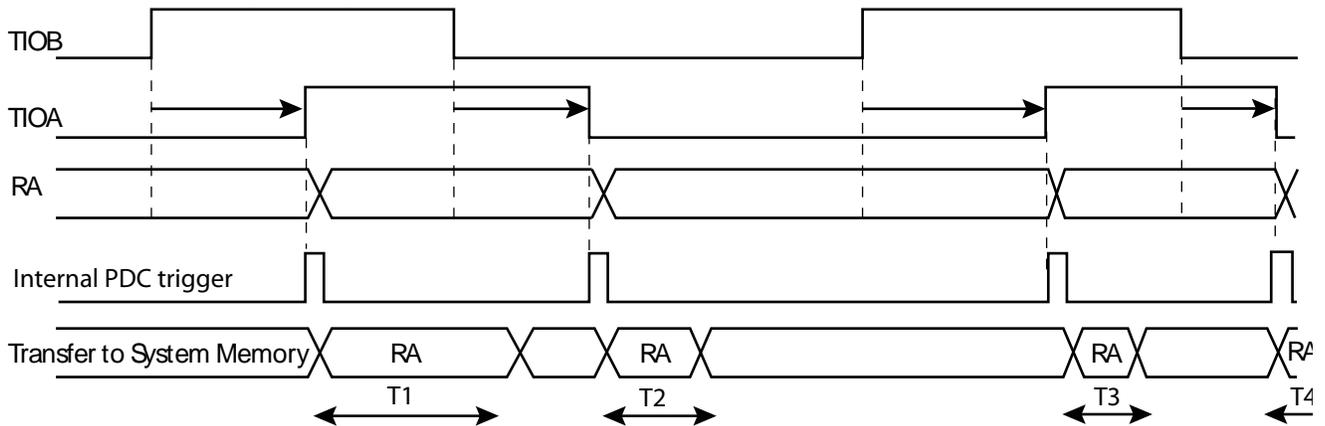
T1,T2,T3,T4 = System Bus load dependent ( $T_{min} = 8 \text{ MCK}$ )
