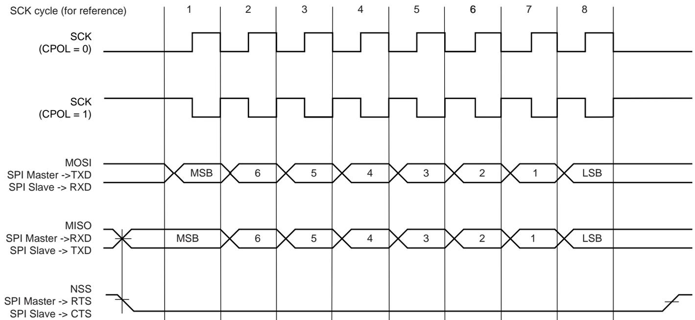
**Figure 35-39. SPI Transfer Format (CPHA=0, 8 bits per transfer)**
