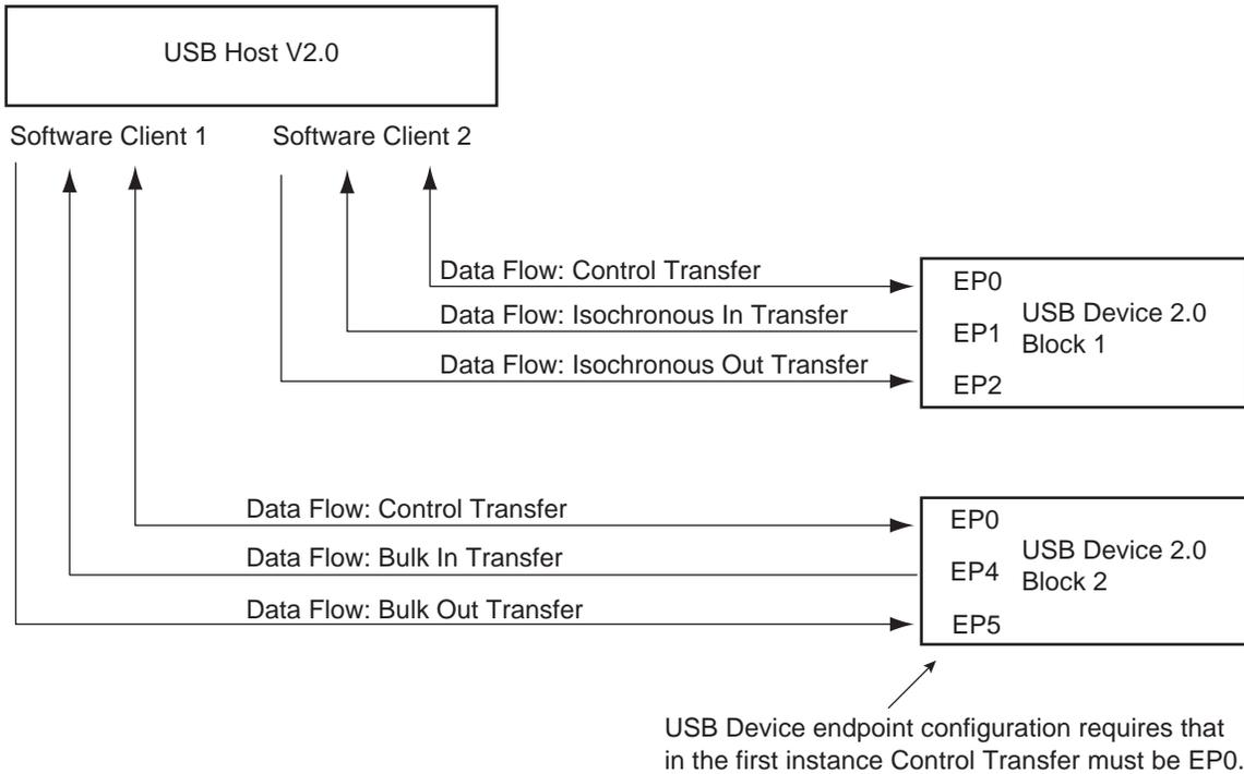
The Control Transfer endpoint EP0 is always used when a USB device is first configured (USB v. 2.0 specifications).
