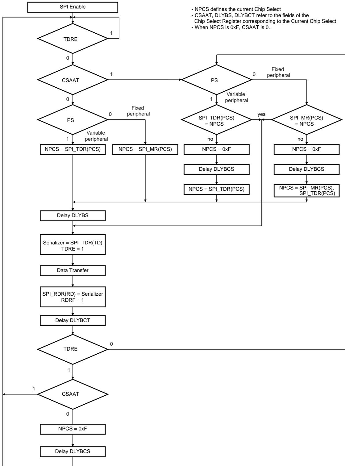
Figure 32-7 shows Transmit Data Register Empty (TDRE), Receive Data Register (RDRF) and Transmission Register Empty (TXEMPTY) status flags behavior within the SPI\_SR (Status Register) during an 8-bit data transfer in fixed mode and no Peripheral Data Controller involved.
