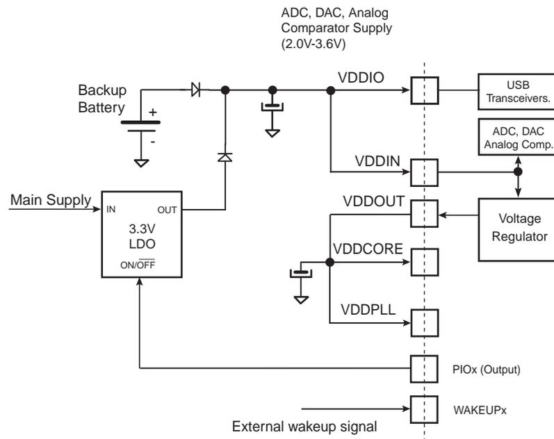
Note: The two diodes provide a “switchover circuit” (for illustration purpose) between the backup battery and the main supply when the system is put in backup mode.
