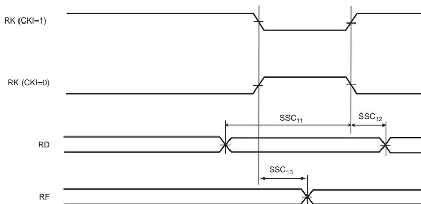
Figure 43-25.SSC Receiver, RK as Output and RF as Input
