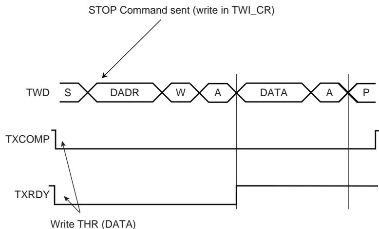
**Figure 33-7. Master Write with Multiple Data Bytes**
