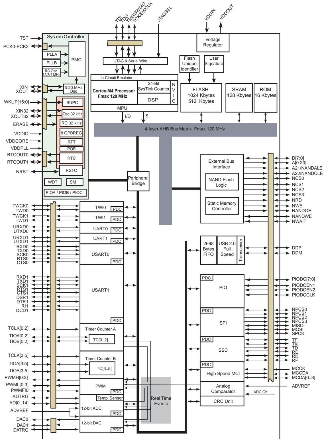
Figure 2-3. SAM4SD32/SD16/SA16 100-pin version Block Diagram
