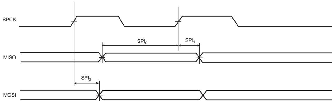
**Figure 43-15. SPI Master Mode with (CPOL = 0 and NCPHA = 1) or (CPOL = 1 and NCPHA = 0)**
