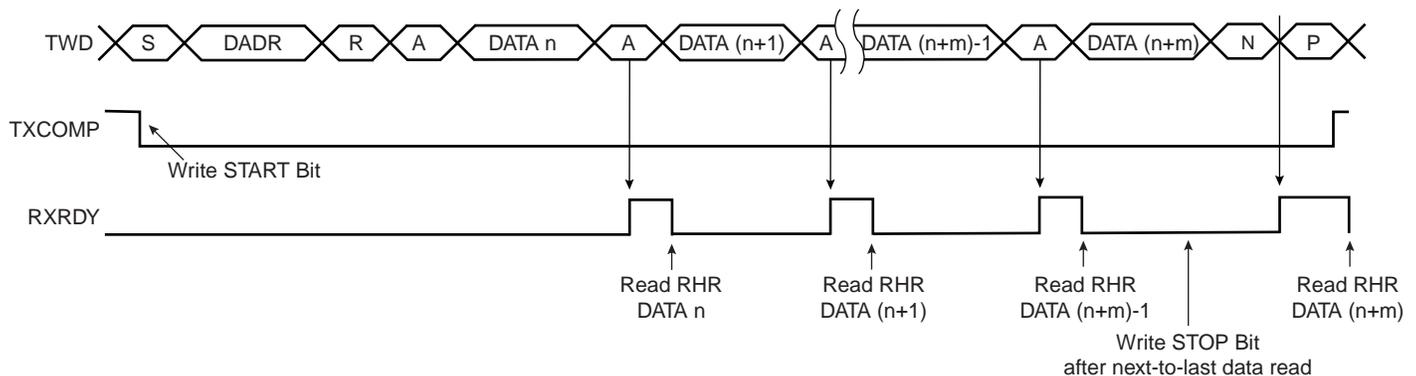
RXRDY is used as Receive Ready for the PDC receive channel.
