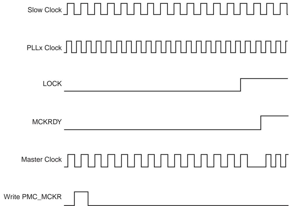
**Figure 28-10. Switch Master Clock from Main Clock to Slow Clock**
