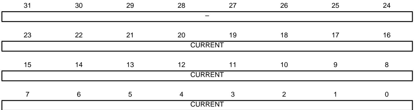
The SysTick SYST\_CVR register contains the current value of the SysTick counter.
