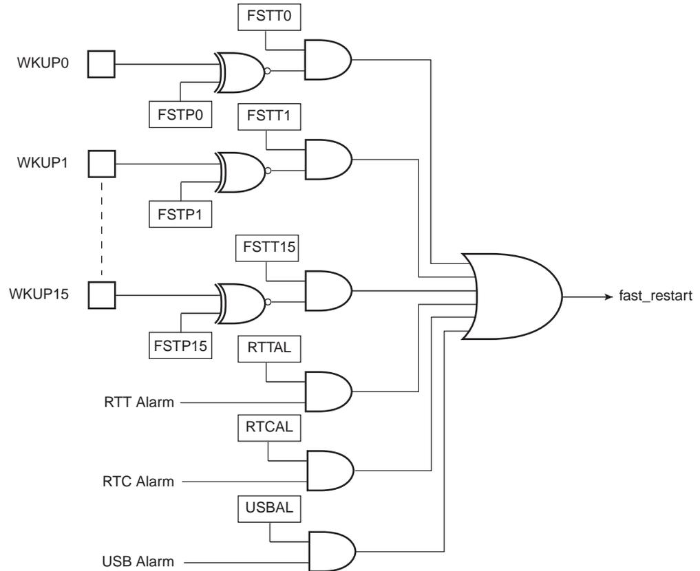
Each wake-up input pin and alarm can be enabled to generate a Fast Start-up event by writing 1 to the corresponding bit in the Fast Start-up Mode Register (PMC\_FSMR).
