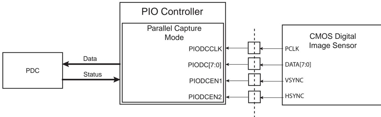
As soon as the parallel capture mode is enabled by writing the PCEN bit at 1 in PIO\_PCMR (“[PIO Parallel Capture Mode Register](#)”), the I/O lines connected to the sensor clock (PIODCCLK), the sensor data (PIODC[7:0]) and the sensor data enable signals (PIODCEN1 and PIODCEN2) are configured automatically as INPUTS. To know which I/O lines are associated with the sensor clock, the sensor data and the sensor data enable signals, refer to the I/O multiplexing table(s) in the product datasheet.
