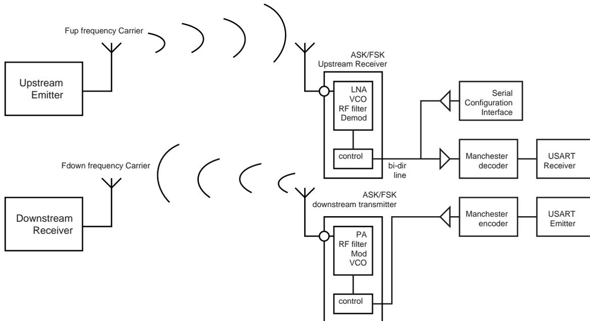
The USART module is configured as a Manchester encoder/decoder. Looking at the downstream communication channel, Manchester encoded characters are serially sent to the RF emitter. This may also include a user defined
