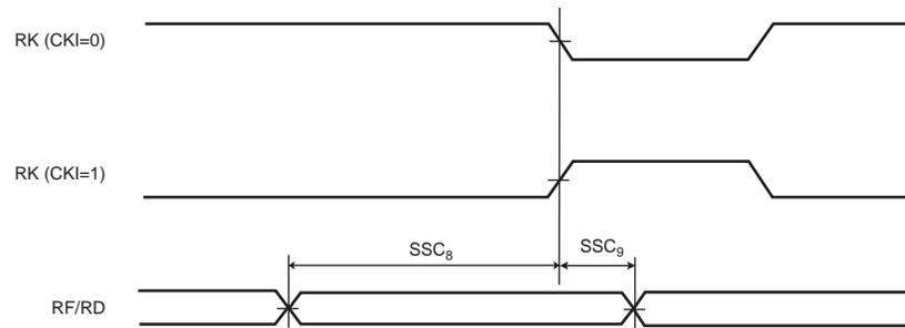
**Figure 43-23.SSC Receiver, RK as Input and RF as Output**
