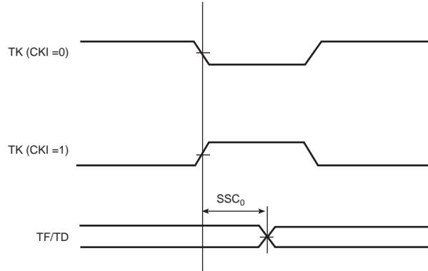
**Figure 43-19.SSC Transmitter, TK as Input and TF as Output**
