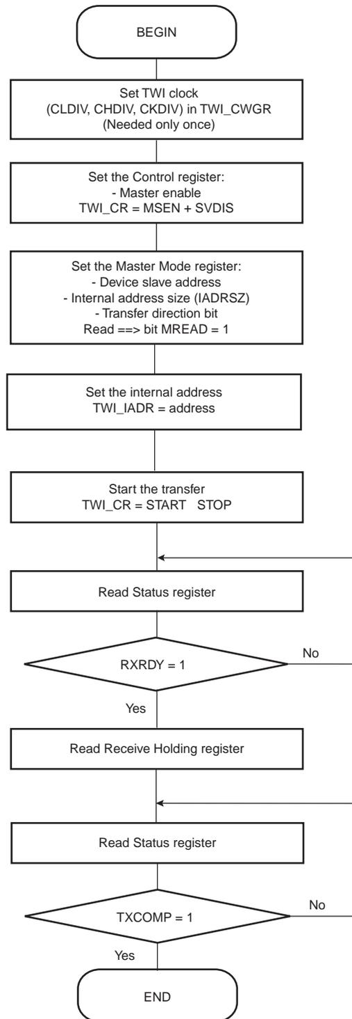
Figure 33-20. TWI Read Operation with Multiple Data Bytes with or without Internal Address
