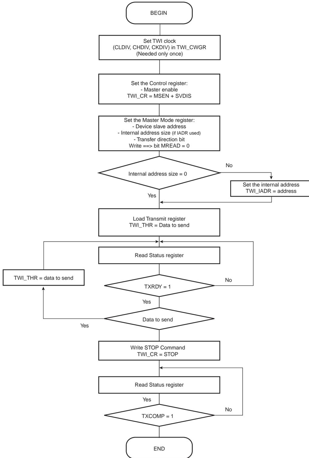
Figure 33-18. TWI Read Operation with Single Data Byte without Internal Address
