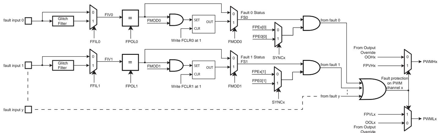
The polarity level of the fault inputs is configured by the FPOL field in the “PWM Fault Mode Register” (PWM\_FMR). For fault inputs coming from internal peripherals such as ADC, Timer Counter, to name but a few, the polarity level must be FPOL = 1. For fault inputs coming from external GPIO pins the polarity level depends on the user's implementation.
