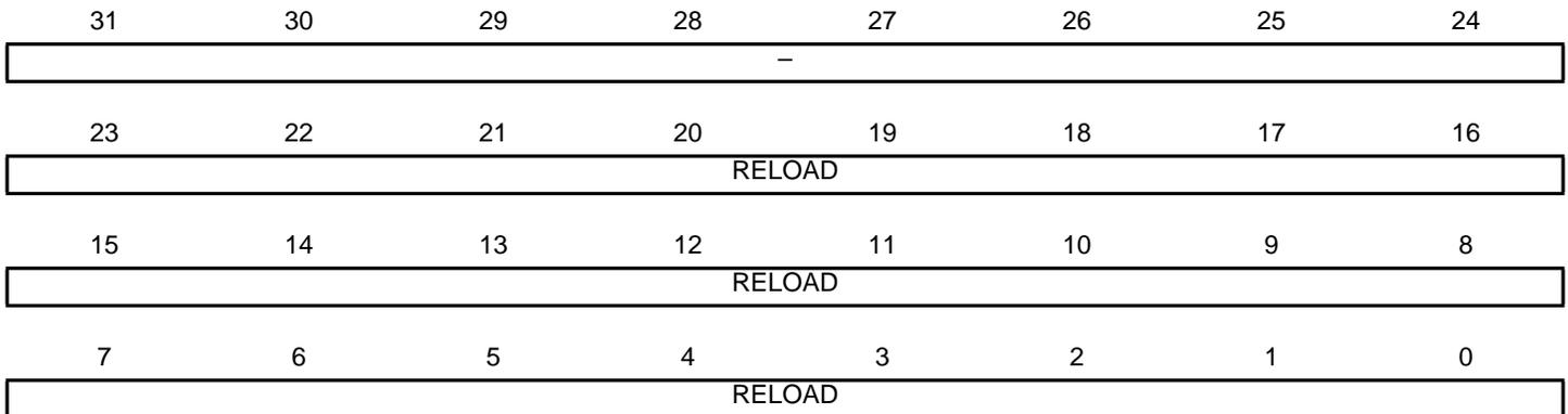
The SYST\_RVR register specifies the start value to load into the SYST\_CVR register.
