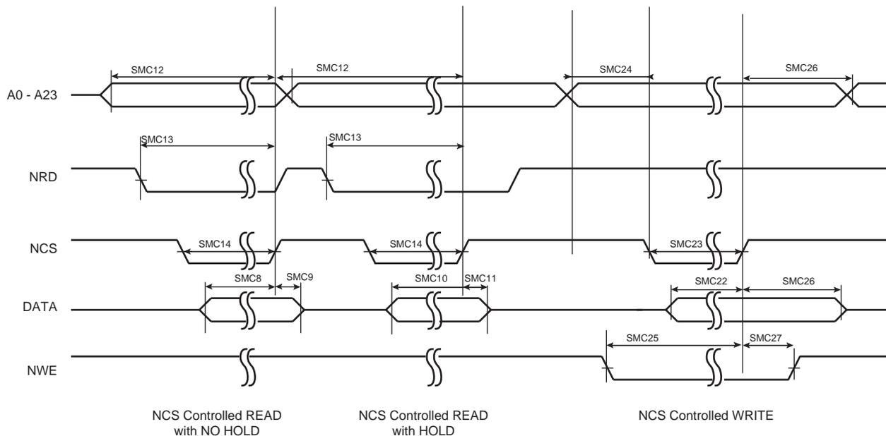
**Figure 43-28.SMC Timings - NRD Controlled Read and NWE Controlled Write**
