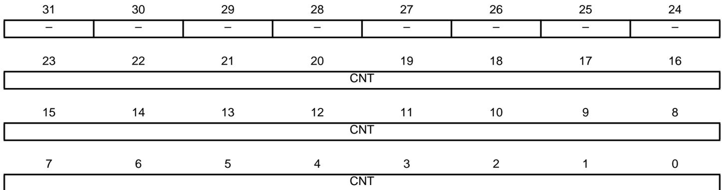
Only the first 16 bits (channel counter size) are significant.
