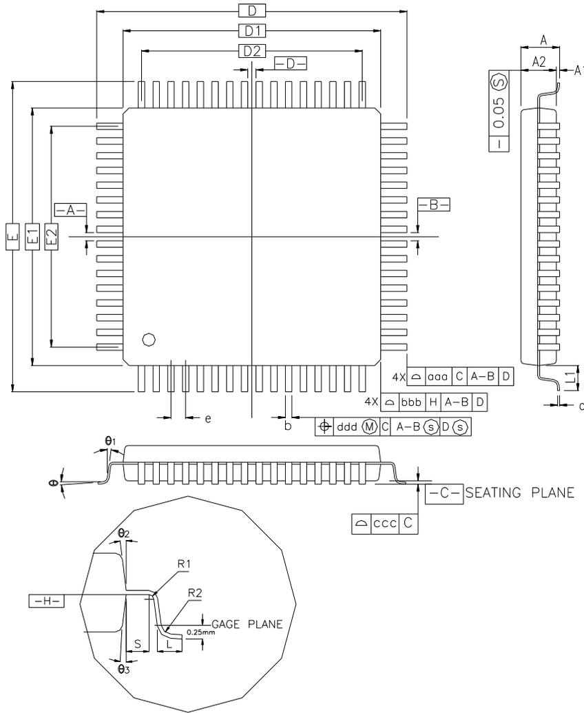
COTROL DIMENSIONS ARE IN MILLIMETERS.
