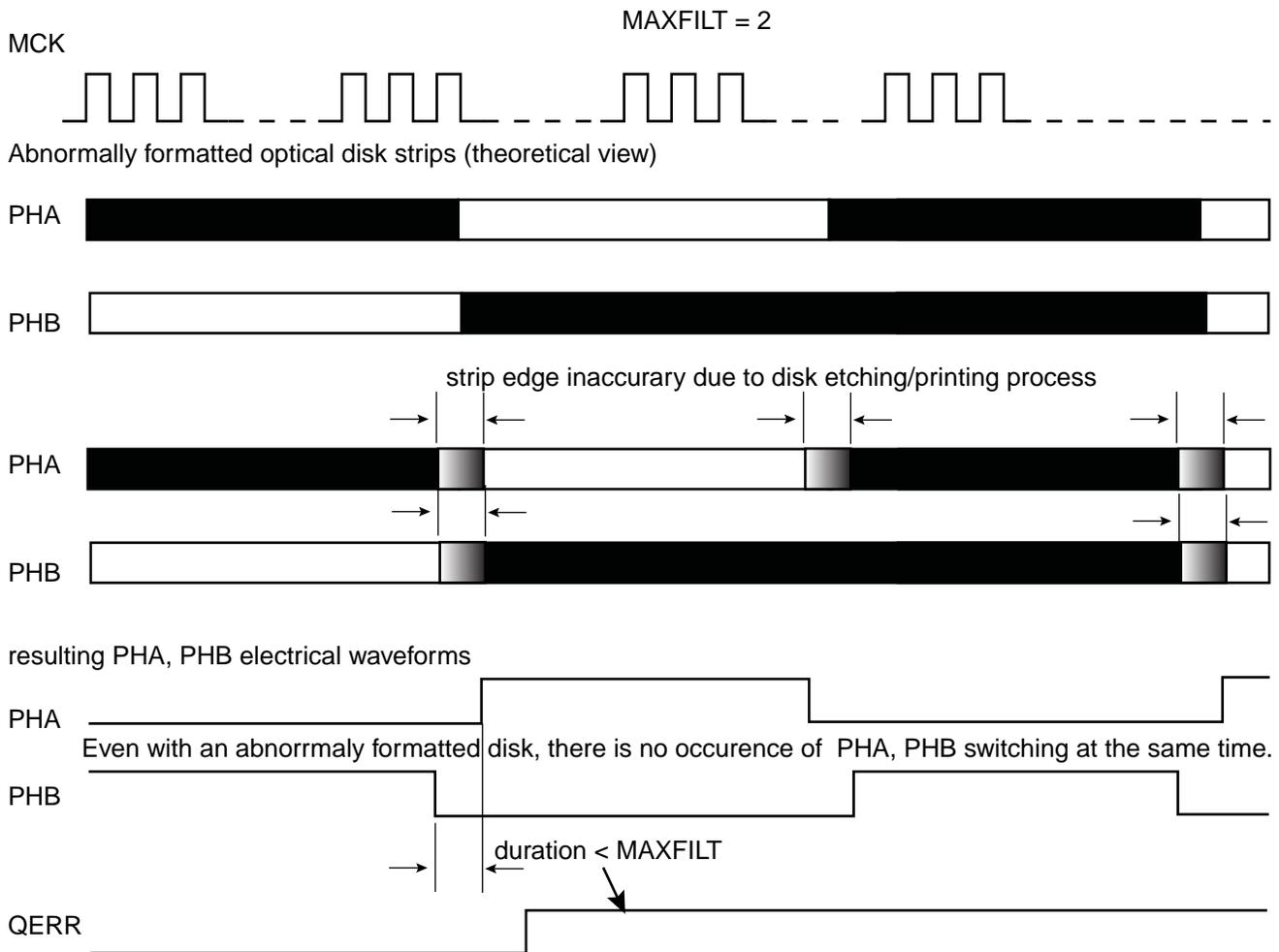
MAXFILT must be tuned according to several factors such as the system clock frequency (MCK), type of rotary sensor and rotation speed to be achieved.
