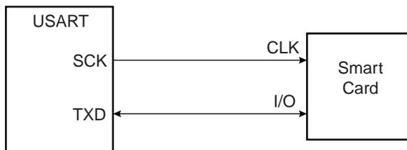
When operating in ISO7816, either in T = 0 or T = 1 modes, the character format is fixed. The configuration is 8 data bits, even parity and 1 or 2 stop bits, regardless of the values programmed in the CHRL, MODE9, PAR and CHMODE fields. MSBF can be used to transmit LSB or MSB first. Parity Bit (PAR) can be used to transmit in normal or inverse mode. Refer to “USART Mode Register” on page 729 and “PAR: Parity Type” on page 730.
