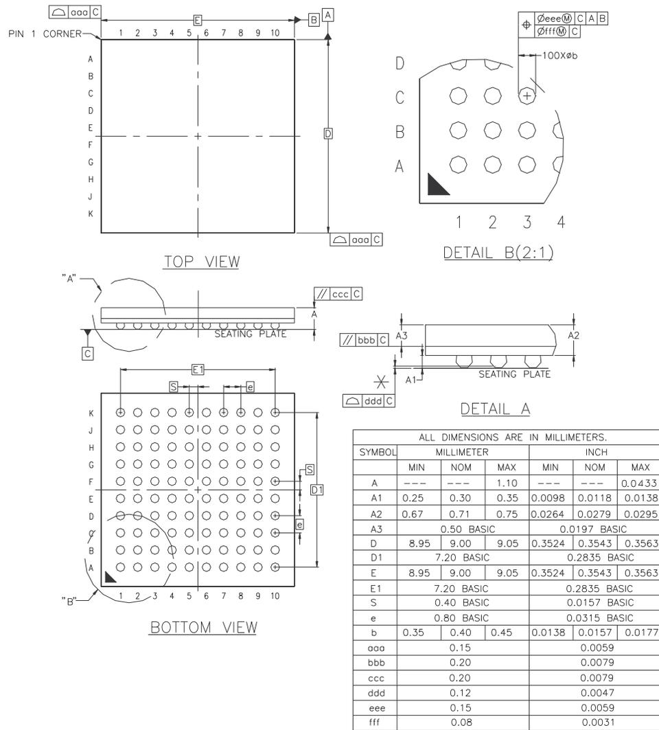
**Table 44-4. TFBGA Package Reference - Soldering Information (Substrate Level)**
