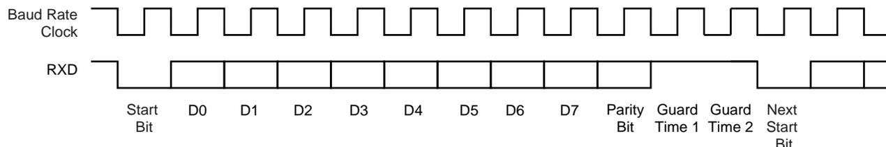
**Figure 35-32. T = 0 Protocol with Parity Error**
