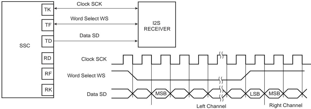
Figure 31-18. Codec Application Block Diagram
