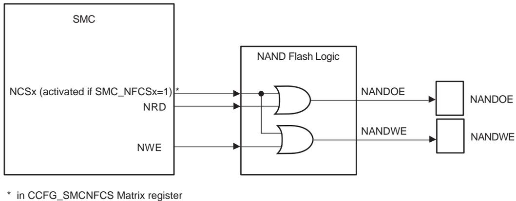
**Note:** When NAND Flash logic is activated, (SMCNFCSx=1), NWE pin cannot be used in PIO Mode but only in peripheral mode (NWE function). If NWE function is not used for other external memories (SRAM, LCD), it must be configured in one of the following modes.
