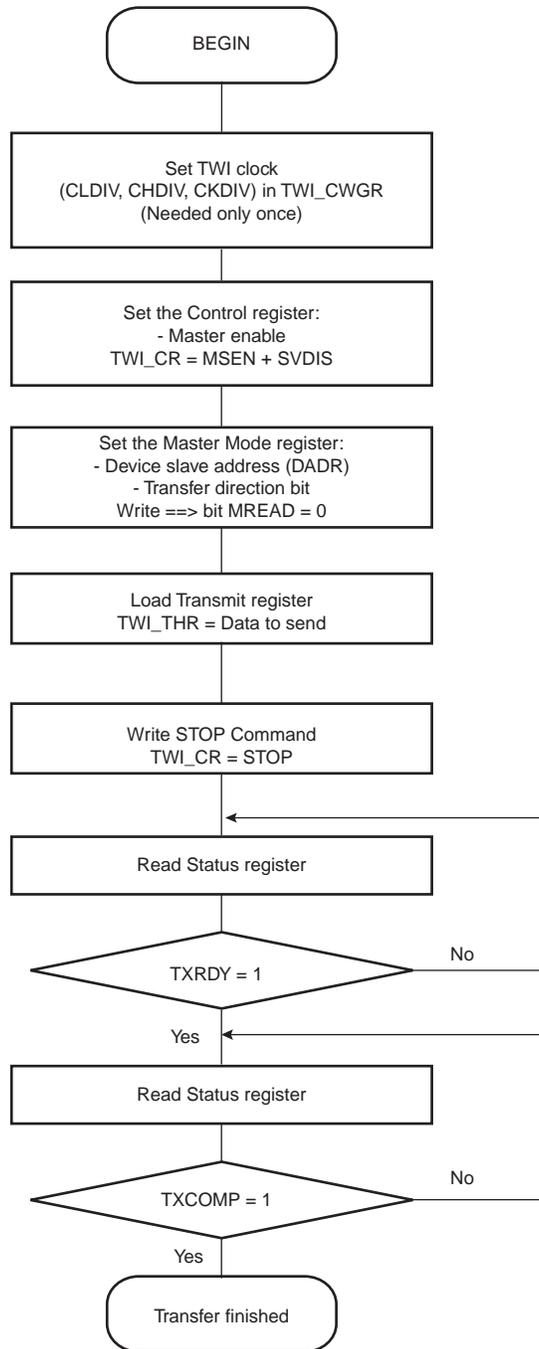
Figure 33-16. TWI Write Operation with Single Data Byte and Internal Address
