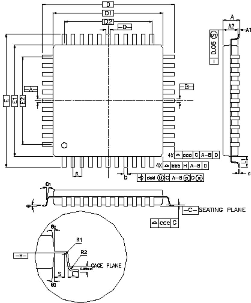
**Table 44-12. 64-lead LQFP Package Dimensions (in mm)**
