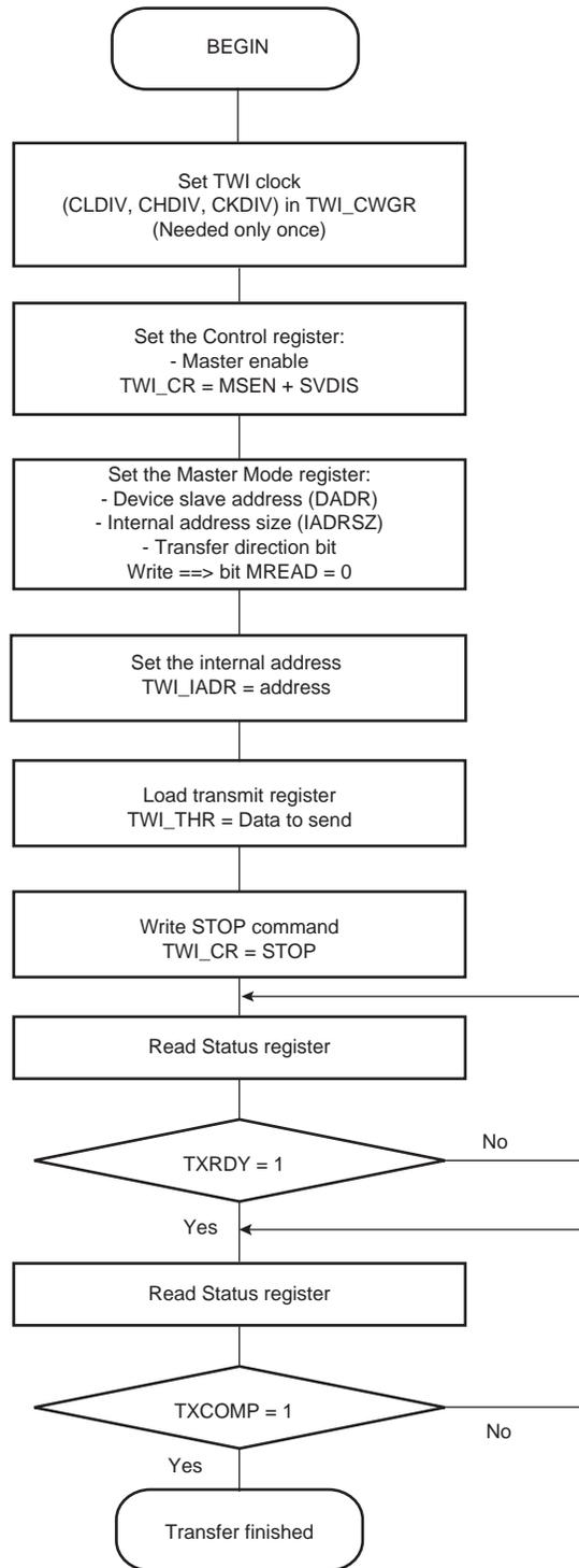
Figure 33-17. TWI Write Operation with Multiple Data Bytes with or without Internal Address
