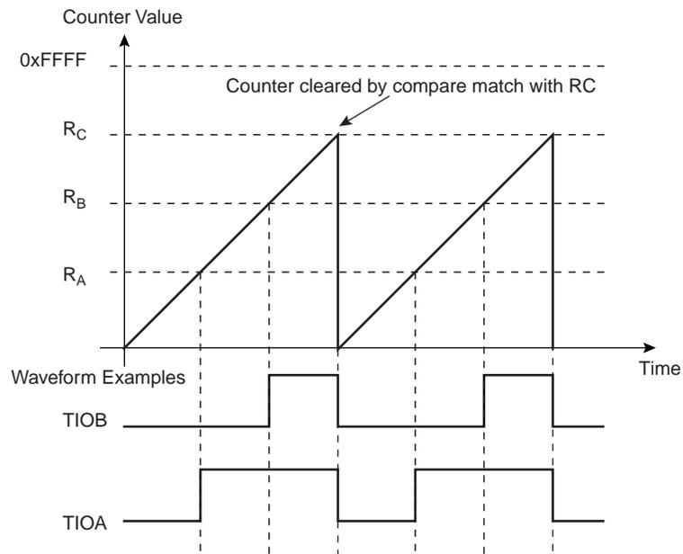
**Figure 36-10. WAVSEL = 10 With Trigger**
