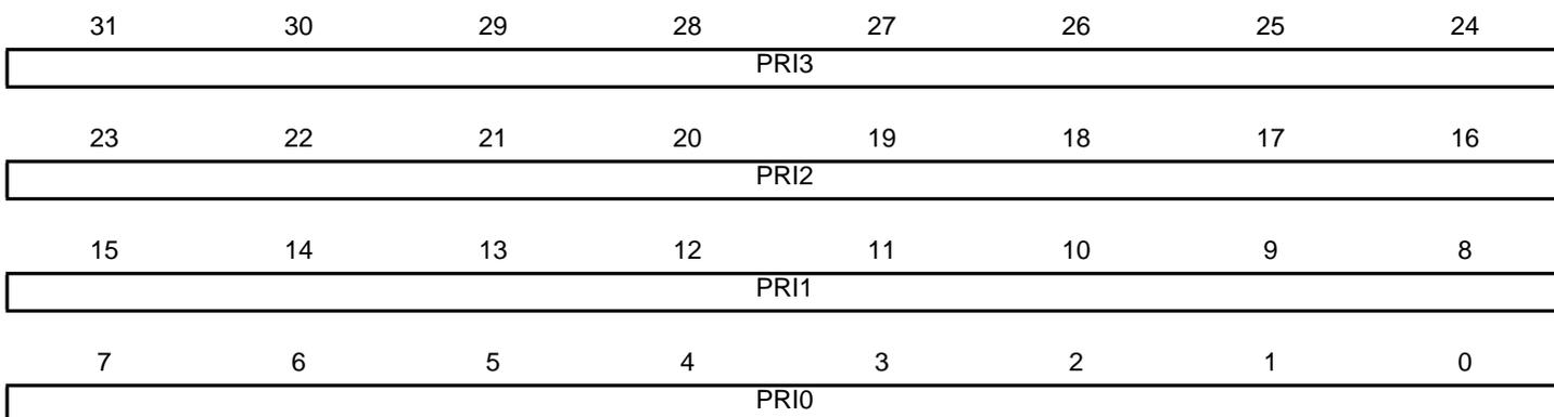
The NVIC\_IPR0-NVIC\_IPR8 registers provide a 4-bit priority field for each interrupt. These registers are byte-accessible. Each register holds four priority fields, that map up to four elements in the CMSIS interrupt priority array IP[0] to IP[34]
