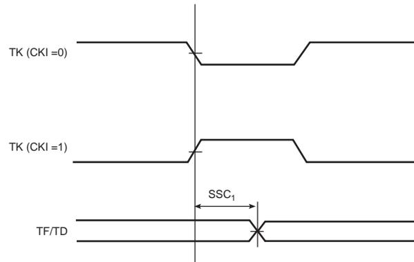
**Figure 43-20.SSC Transmitter, TK as Output and TF as Input**
