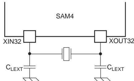
$$C_{LEXT} = 2X(C_{CRYSTAL} - C_{para} - C_{PCB}).$$
