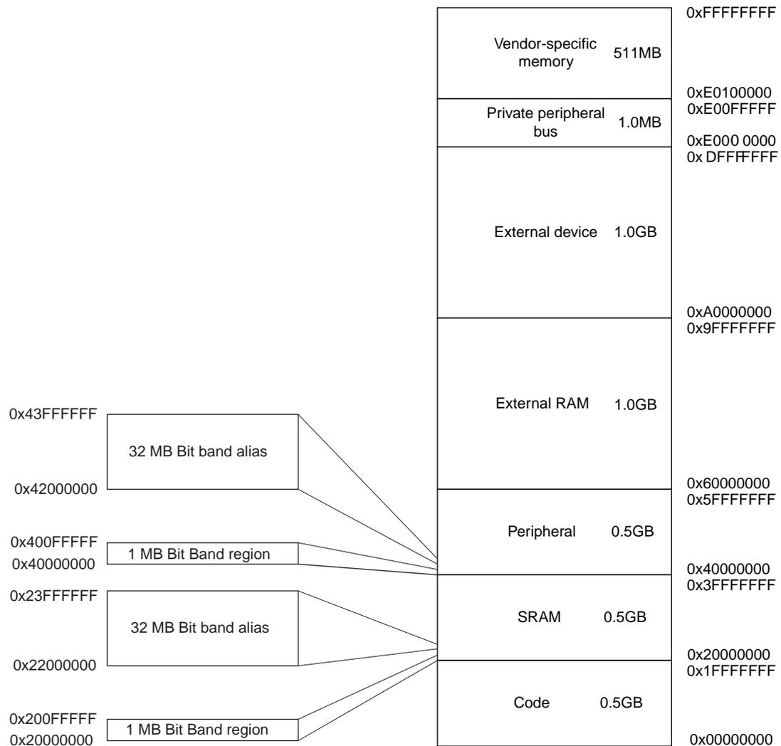
The regions for SRAM and peripherals include bit-band regions. Bit-banding provides atomic operations to bit data, see [“Bit-banding”](#).
