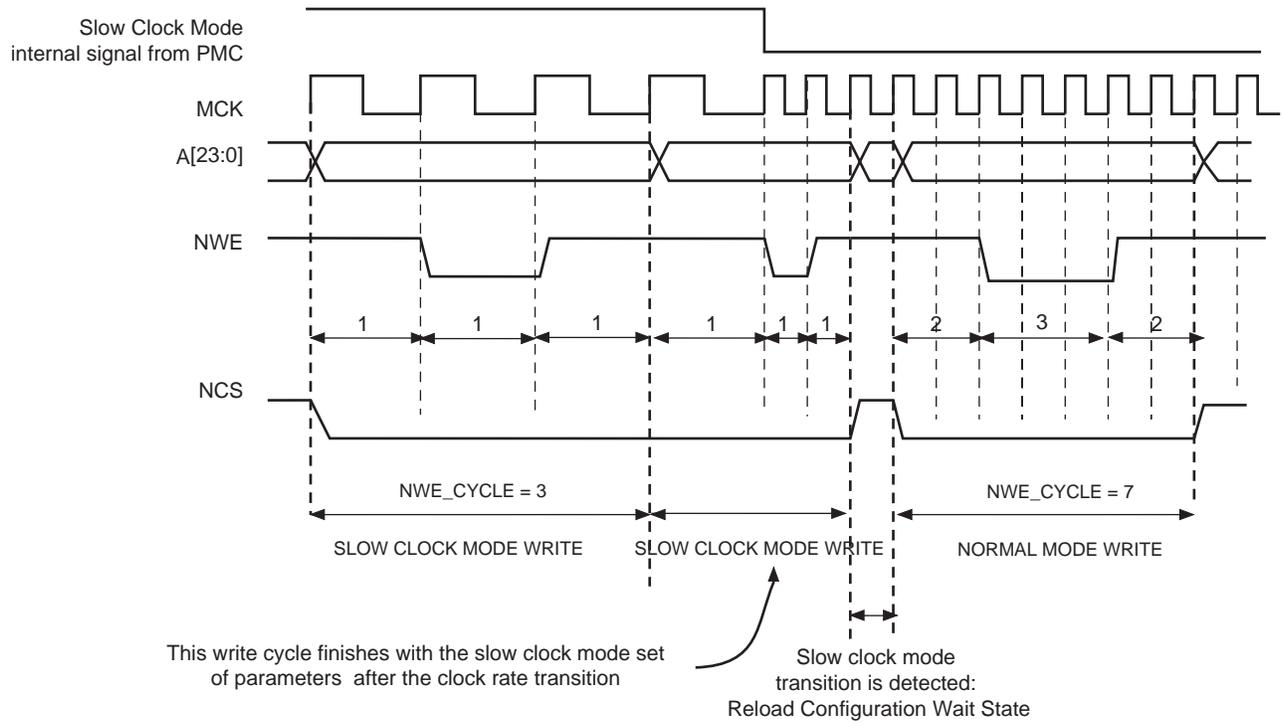
**Figure 26-30. Recommended Procedure to Switch from Slow Clock Mode to Normal Mode or from Normal Mode to Slow Clock Mode**
