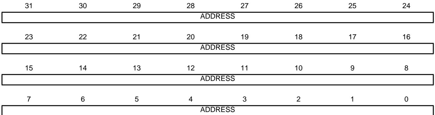
The BFAR register contains the address of the location that generated a bus fault.
