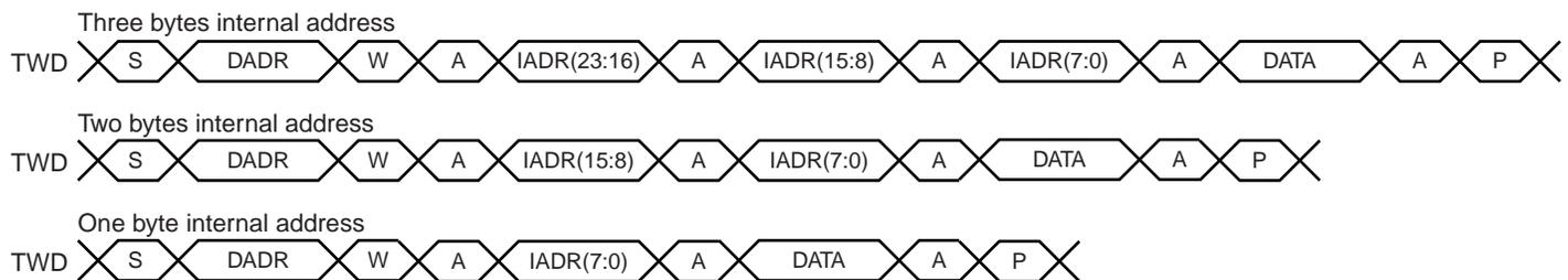
**Figure 33-12. Master Read with One, Two or Three Bytes Internal Address and One Data Byte**
