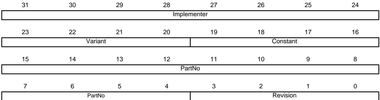
The SCB\_CPUID register contains the processor part number, version, and implementation information.
