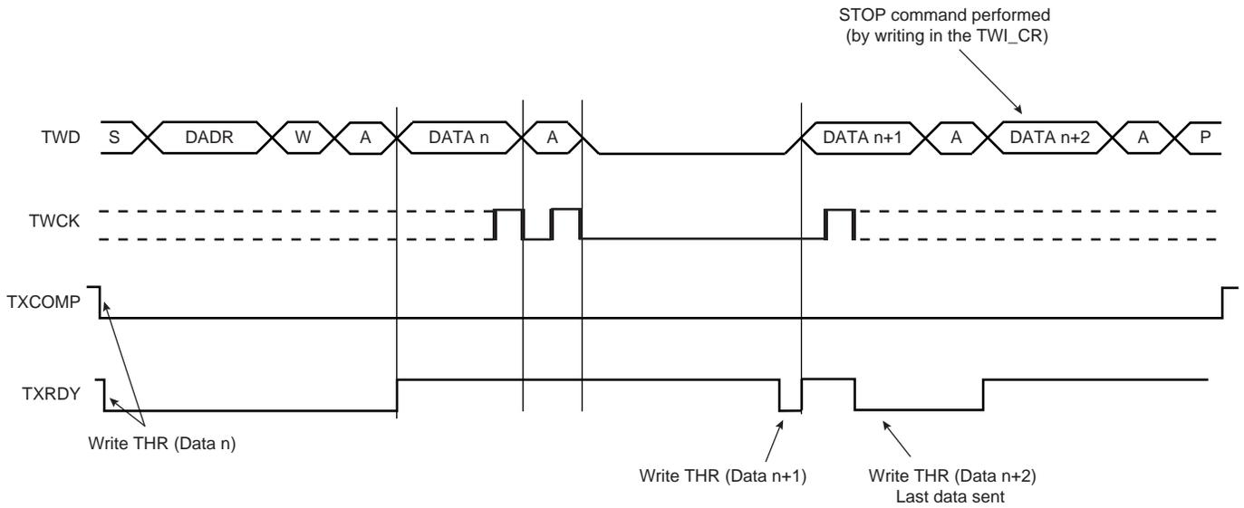
**Figure 33-8. Master Write with One Byte Internal Address and Multiple Data Bytes**
