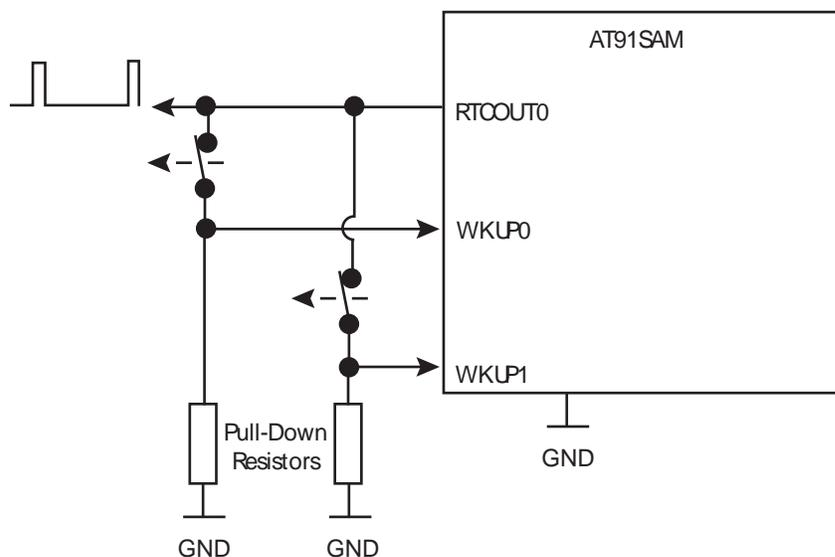
The debouncing parameters can be adjusted and are shared (except the wake up input polarity) by both debouncers. The number of successive identical samples to wake up the core can be configured from 2 up to 8 in the LPDBC field of SUPC\_WUMR. The period of time between 2 samples can be configured by programming the TPERIOD field in the RTC\_MR register.
