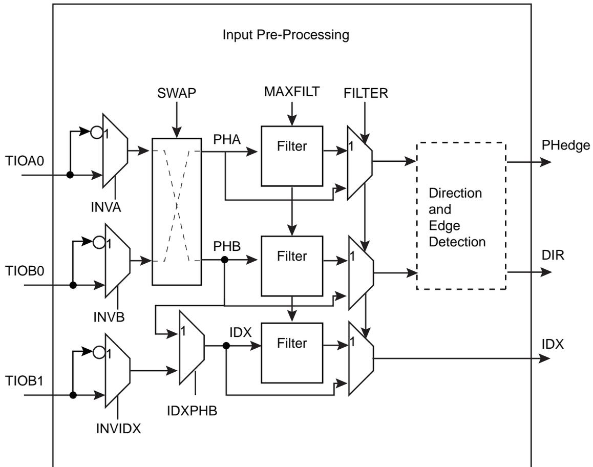
Input filtering can efficiently remove spurious pulses that might be generated by the presence of particulate contamination on the optical or magnetic disk of the rotary sensor.
