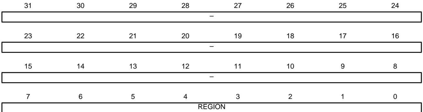
The MPU\_RNR selects which memory region is referenced by the MPU\_RBAR and MPU\_RASR registers.
