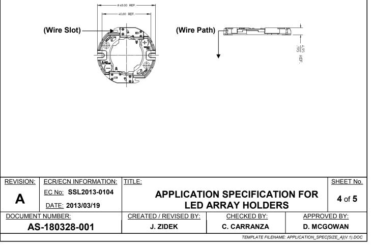
5.0.6 - Thread wires through the two original wire path holes in the heat sink/fixture
