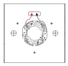
5.0.7 – Pull wires through holes ensuring that the holder is placed and fits flush on the top of the heat sink or with the mounting area on the inside of the fixture
