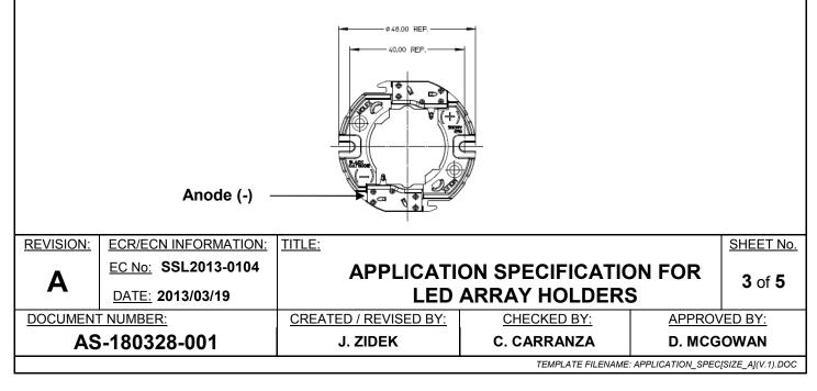
5.0.4 – Insert the red wire into the indicate cathode (+) wire trap slot
