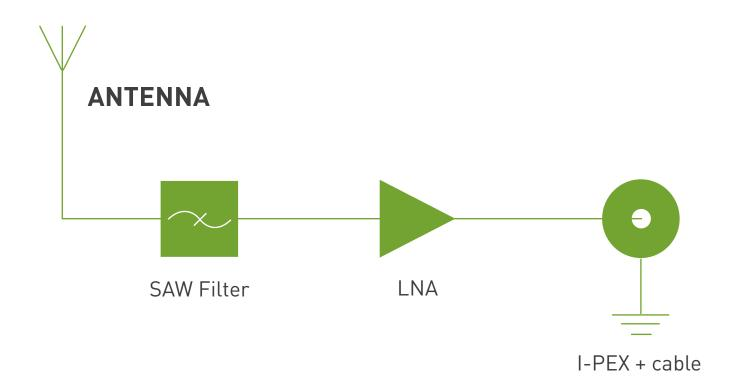
The AP.25E has a SAW filter on the front of it. The main use of the AP.25E would be for small devices where the GSM transmitter is close to the GPS antenna, it helps avoid
