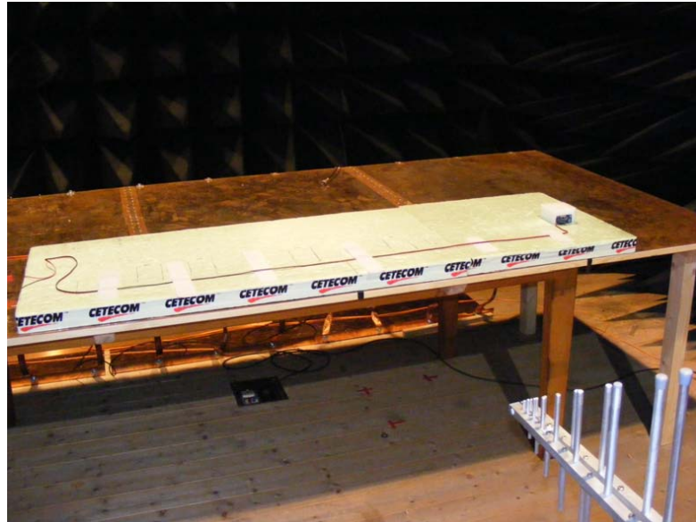
Photo 2: Emission Stripline 500 kHz - 1000 MHz
