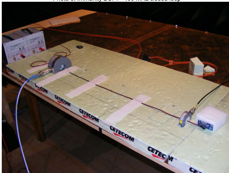
Photo 6: Immunity BCI 1 - 400 MHz closed loop
