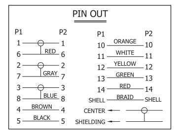
1.CABLE:28AWG(7/0.127 T.C)\*3COAX(75 OHMS)+INSULATION:FO-PE INNER JACKET:PVC OD:Ø2.5± 0.1mm(UL-1354)+28AWG(7/0.127 T.C)\*7C+ INSULATION:SR-PVC ID:Ø0.85± 0.05mm(UL-1061)+AL/MY+DRAIN WIRE:26AWG(7/0.16 T.C)+BRAID SHIELD(85%)+OUTER JACKET:PVC COLOR:BEIGE,OD:Ø8.5± 0.15mm UL-2919
