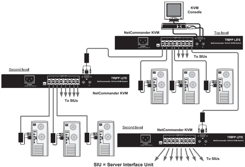
Figure 5.9 Cascading NetCommander KVM Switches
