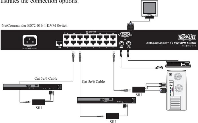
Figure 5.4 NetCommander KVM system connections
