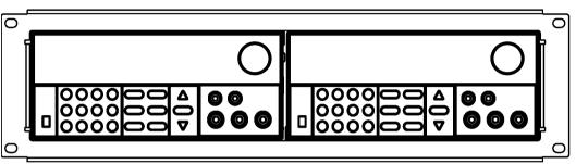
To rack mount two instruments (models 9120A, 9121A, 9122A, 9123A, 9124 only) side-by-side, order rack mount kit IT-E151, In this case you don't need to use the front cover panel.
