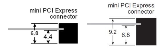
The SMT connectors are ideal in a development environment, where the latch connector facilitates swapping ConnectCard for i.MX28 modules as development progresses. The absence of holes also maximizes trace routing flexibility on the printed circuit board. The standoff option offers better vibration resistance and grounding once you are ready to deploy your application based on the ConnectCard for i.MX28.
