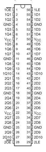
A buffered output-enable (1OE or 2OE) input can be used to place the outputs of the corresponding 10-bit latch in either a normal logic state (high or low logic levels) or a high-impedance state. In the high-impedance state, the outputs neither load nor drive the bus lines significantly.
