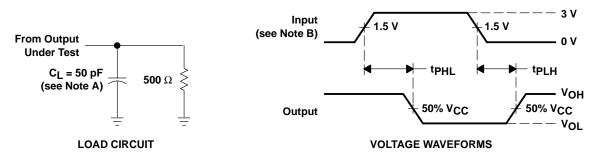
NOTES: A. C<sub>L</sub> includes probe and jig capacitance.
