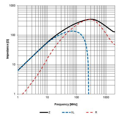
Test Equipment: E4991A or equivalent
