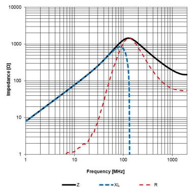
Test Equipment: E4991A or equivalent
