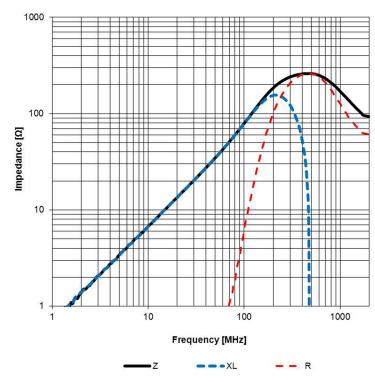
Test Equipment: E4991A or equivalent
