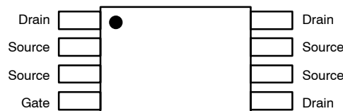
Figure 2. Pinouts for Single Die TSSOP
