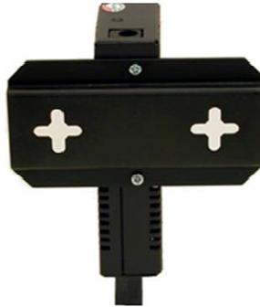
The IE-MultiWay can be mounted with two DIN Rail clips, a hardware option available through IMC Networks. The DIN Rail clips include screws, to allow the installation onto a DIN Rail. Install the screws into DIN Rail clips, which can be mounted parallel or perpendicular to the DIN Rail. Snap the converter onto the clips. To remove the converter from the DIN Rail, use a flat-head screwdriver into the slot to gently pry the converter from the rail. Refer to picture on page 7.
