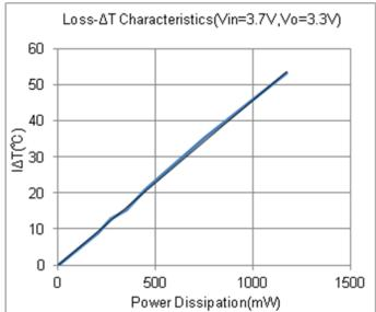
The output current of the device may need to be de-rated if it is operated in high ambient temperature or in an application that requires continuous power delivery. The amount of current de-rating is highly dependent on the environmental thermal conditions, e.g., PCB design, nearby components or effective air flows. Care should especially be taken in applications where the device temperature exceeds 85°C.
