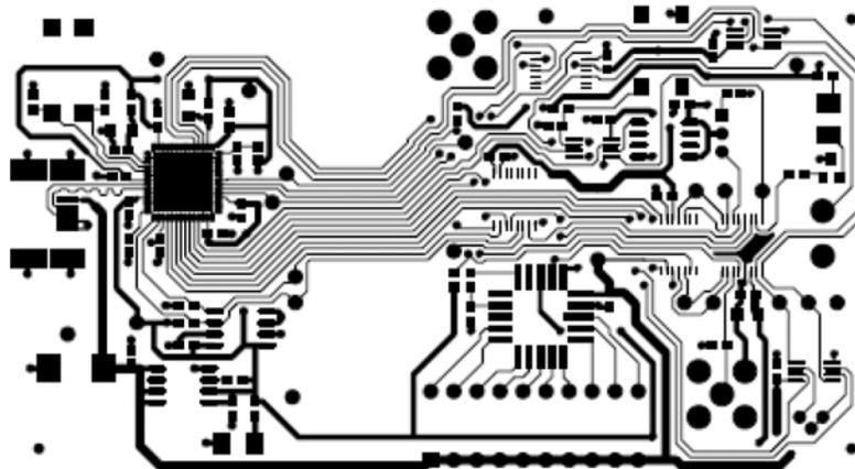
Figure 20. ADT7516 Evaluation Board PCB Layout (Component Side)
