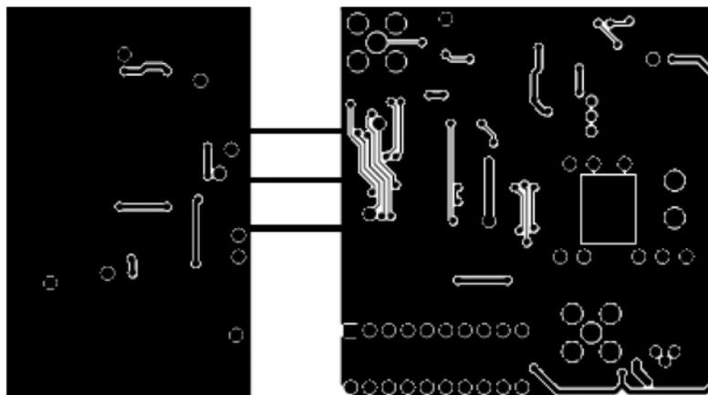
Figure 21. ADT7516 Evaluation Board PCB Layout (Solder Side)
