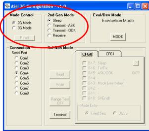
Transmitting using 2G Mode requires applying an external signal to the TX testpoint terminal from a user application or function generator. Received data may be viewed by connecting an oscilloscope probe to the RX testpoint terminal or connecting to a user application.
