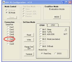
Click READ on each device and make sure that the synthesizer is locked. This should read out a 0x0040, but may depend on the previous power-up state. As long as bit 6 of the CFG1 register is checked, the synthesizer is locked.
