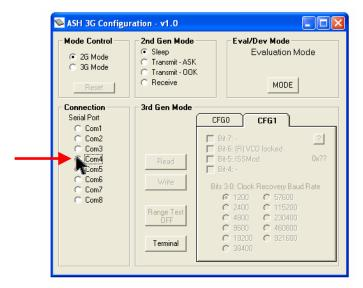
After selecting the COM port, turn on the development board. The LED's should light in sequence and the "Heartbeat" will flash.
