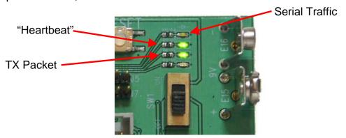
On the receiver board two LED's will flash continuously. The "CRC Good" LED flashes when the packet is received and the frame check (CRC) of the packet has been verified as good and the "Serial Traffic" LED will flash when an ACK or nACK is sent to the PC via the serial port. The ACK or nACK will appear in the Transmit window of the configuration software.
