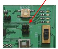
To disable Range Test, switch SW1 to **OFF**, remove jumper, switch SW1 back to **ON** to power the board.
