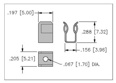
Material: .016 [0.40] Brass, Tin Plate Current Rating: 10 Amps
