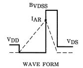
$$\begin{array}{l} T_{ch} = 25^{\circ}C \text{ (Initial)} \\ \text{Peak I}_{AR} = 5 \text{ A, R}_{G} = 25 \ \Omega \\ \text{V}_{DD} = 16 \text{ V, L} = 1.0 \text{ mH} \end{array} \\ \text{EAS} = \frac{1}{2} \cdot \text{L} \cdot \text{I}^{2} \cdot \text{(} \frac{\text{BVDSS}}{\text{BVDSS} - \text{V}_{DD}} \text{)} \\ \end{array}$$
