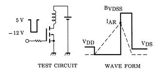
$$\begin{array}{l} T_{ch} = 25^{\circ}\!C~(Initial) \\ Peak~I_{AR} = -6~A,~R_G = 25~\Omega~~E_{AS} = \frac{1}{2} \cdot L~\cdot I^2~\cdot~(\frac{BVDSS}{BVDSS - V_{DD}}) \\ V_{DD} = -16~V,~L = 1.0~mH \end{array}$$
