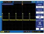
Monitor and analyze long-term signal behavior by recording data continuously over an extensive period of time and playing it back for post acquisition analysis. Data is recorded in a sequence of up to 1000 frames.
