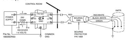
**Grounding:** The 8-32 mounting screw and attached clamp, and hence the DIN-1 (TS-32) or DIN-3 (TS-35) rail, serve as the protector ground. The rail (or 8-32 mounting screw if the clamp is not used) should be connected to the facility ground via an AWG #6 or larger copper wire. This wire should be as short and straight as possible. Single point grounding will provide better protection and will permit the protector to be located a distance from the equipment.
