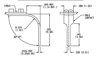
ALL DIMENSIONS: INCHES [MILLIMETERS] ALL TOLERANCES:  $\pm 0.005$  [0.13] UNLESS OTHERWISE SPECIFIED MAY SHIP WITH OR WITHOUT POLARIZATION STRIPE UNLESS SPECIFIED CONSULT FACTORY FOR OTHER SIZES AND CONFIGURATIONS CUSTOMIZATION: ARIES SPECIALIZES IN CUSTOM DESIGN AND PRODUCTION. SPECIAL MATERIALS, PLATINGS, SIZES, AND CONFIGURATIONS CAN BE FURNISHED, DEPENDING ON QUANTITY.
