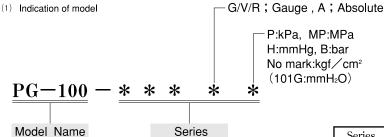
$\begin{array}{lll} \hbox{(2) Type} & \hbox{G/V/R--Gauge pressure, A---Absolute pressure} \\ \hbox{(3) Display} & \hbox{3 1/2 Digits --1999 } \sim 1999 \ \text{max., LCD Digital} \\ \end{array}$
