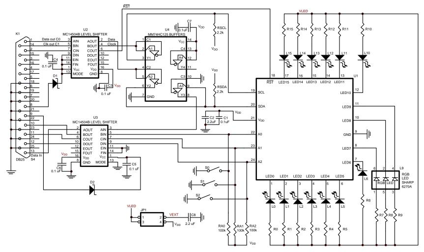
Figure 3. LP3943 Board Schematic
