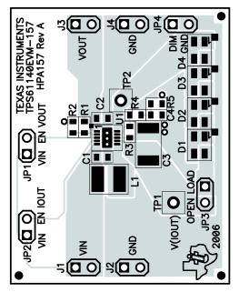
Figure 3. Top Assembly Layer
