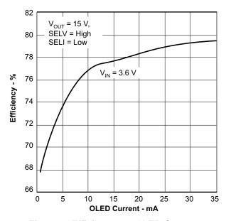
Figure 1. Efficiency vs. WLED Current
