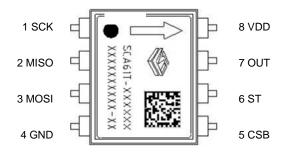
**Figure 3.** SCA61T electrical connection
