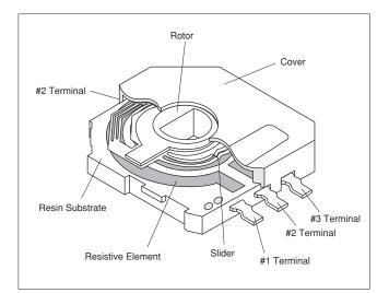
When soldering, take care that the tip of the soldering iron does not come into direct contact with the product (cover, rotor, plastic substrate, etc.).
