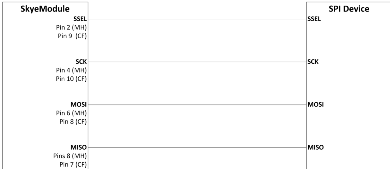
Figure 10-3: SPI Connection Diagram
