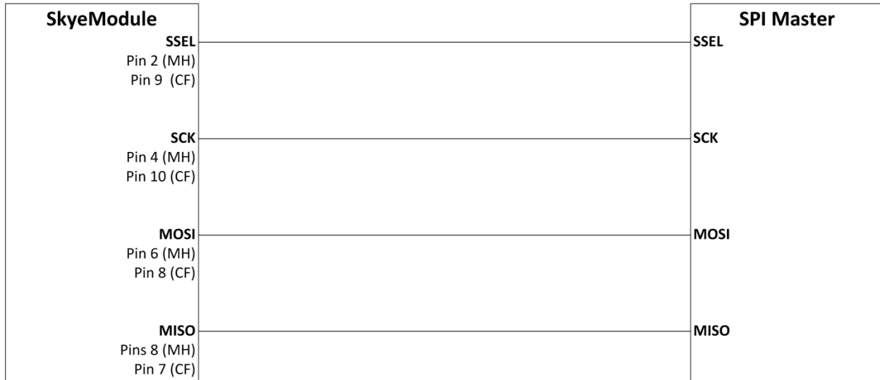
Figure 9-3: SPI Connection Diagram
