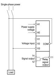
Note: There is no polarity when a DC current input is used.
