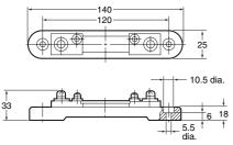
Current terminal: M6 screw Voltage terminal: M4 screw
