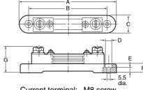
Current terminal: M8 screw Voltage terminal: M4 screw
