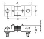
Current terminal: M12 screw Voltage terminal: M5 screw
