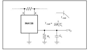
FIGURE 2. Buffering Output to Drive an A/D Converter.
