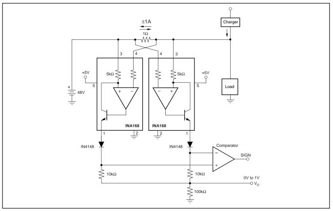
FIGURE 5. Bipolar Current Measurement.
