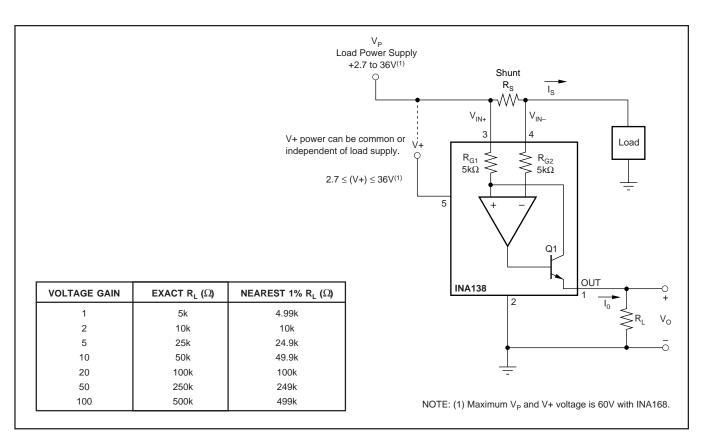
FIGURE 1. Basic Circuit Connections.
