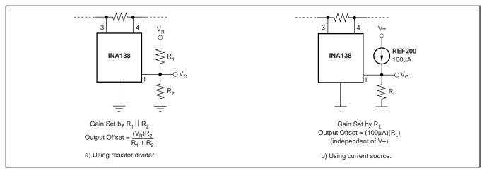
FIGURE 4. Offsetting the Output Voltage.
