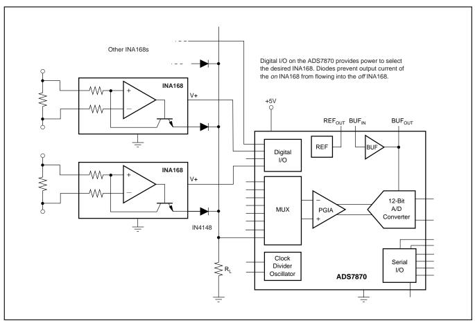
FIGURE 7. Multiplexed Measurement Using Logic Signal for Power.
