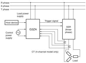
Note: Connect to one of the three phases on the load power supply input terminals of the G3ZA.
