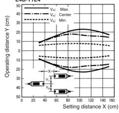
Note: Obtain the point that turns Y<sub>1</sub> and Y<sub>2</sub> ON while changing the sensing distance (X).
