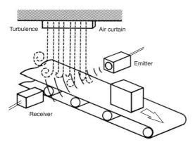
The jetting sound of air nozzles includes noise of a wide frequency range, which will affect the operation of the E4B. Do not use an air nozzle near the E4B.
