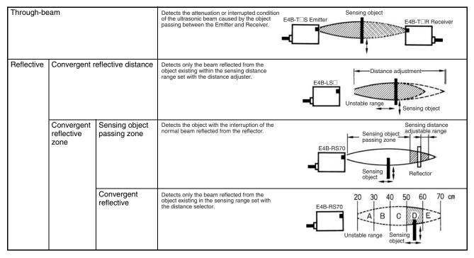
**Note:** An object may be detected due to multiple reflection if the object is in the unstable range where the distance adjuster is ineffective, in which case however, the detection of the object will not be stable. Therefore, do not attempt to use the E4B to detect an object in the unstable range.
