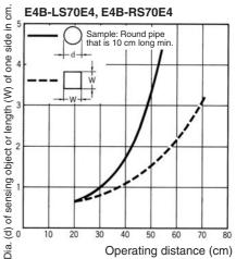
Note: The curve with the sensitivity adjuster set to maximum indicates the size of the sensing object.
