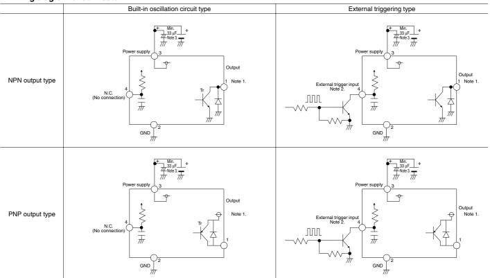
Notes: 1. The output transistor has an open collector structure.
