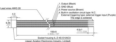
Note: Mistaken cable assembly can cause damage to the internal circuits, so please check the power cord before switching ON. (Particular care must be taken as to avoid reverse connection of the power.)
