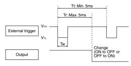
Note: The sensor recognizes at the  $V_{TH} \rightarrow V_{TL}$  edge of an external trigger that the external trigger has been input.
