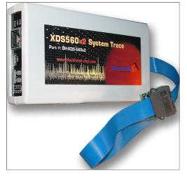
ribbon coax JTAG cable. The XDS560v2 adds support for IEEE1149.7 and the system trace module (STM), an interface on the TI heterogeneous multi-core (ARM + DSP) devices. If you are familiar with the Blackhawk LAN560 product, you will already be familiar with this new design.
