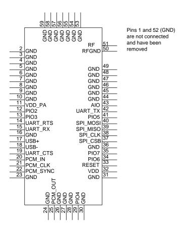
Figure 1: WT41 pin out
