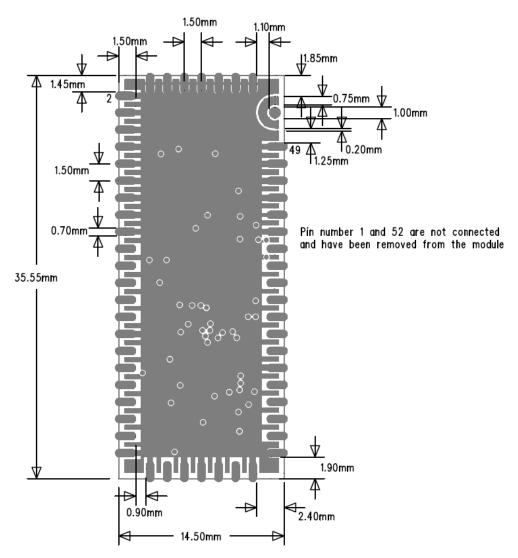
Figure 2: Physical dimensions (top view)
