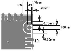
Figure 3: Dimensions for the RF pin (top view)
