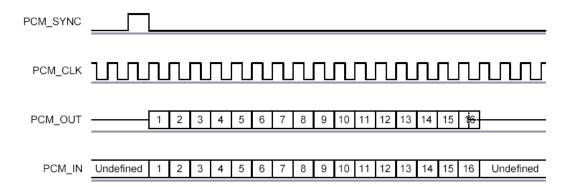
Figure 16: Short Frame Sync (Shown with 16-bit Sample)
