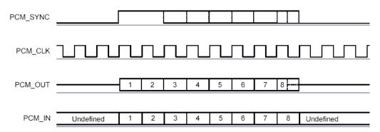
Figure 15: Long Frame Sync (Shown with 8-bit Companded Sample)
