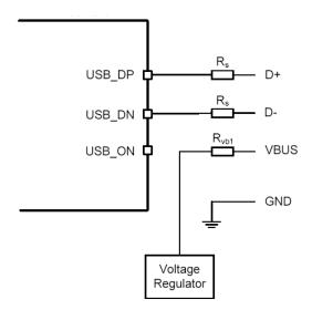
Figure 11: USB Connections for Bus-Powered Mode
