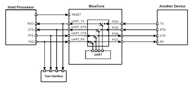
Figure 8: UART Bypass Architecture
