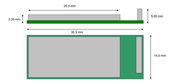
Figure 4: Dimensions of WT41
