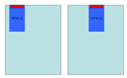
Figure 6: Recommended positions for WT41-A
