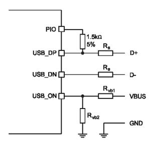
Figure 9: USB Connections for Self-Powered Mode
