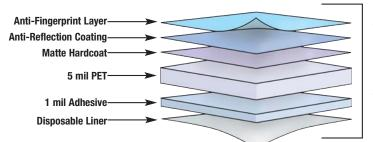
Vikuiti Removable Anti-Reflection Film's unique multilayered construction reduces glare, makes it easier to wipe off fingerprints and helps shield screens from scratches.
