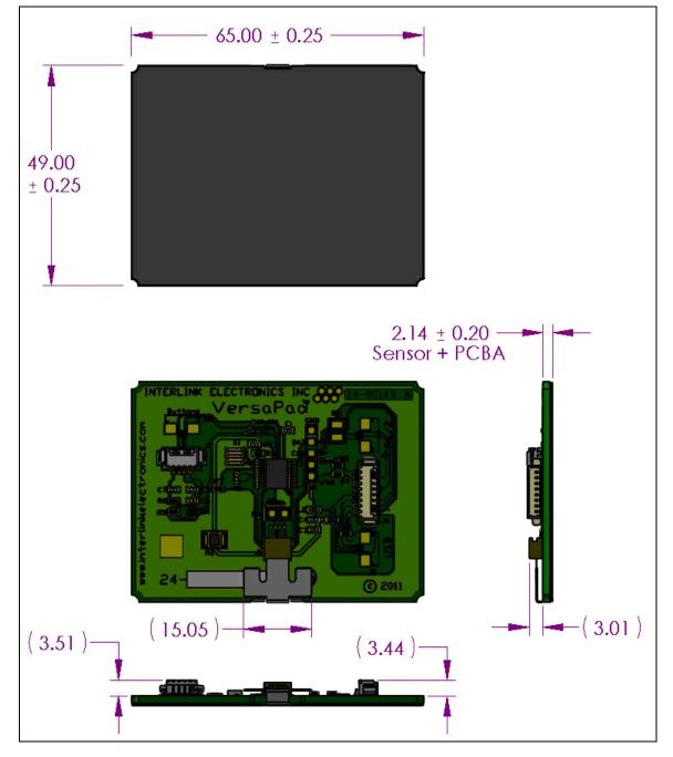
Figure 12: Overall dimensions of VersaPad. All dimensions are in mm.
