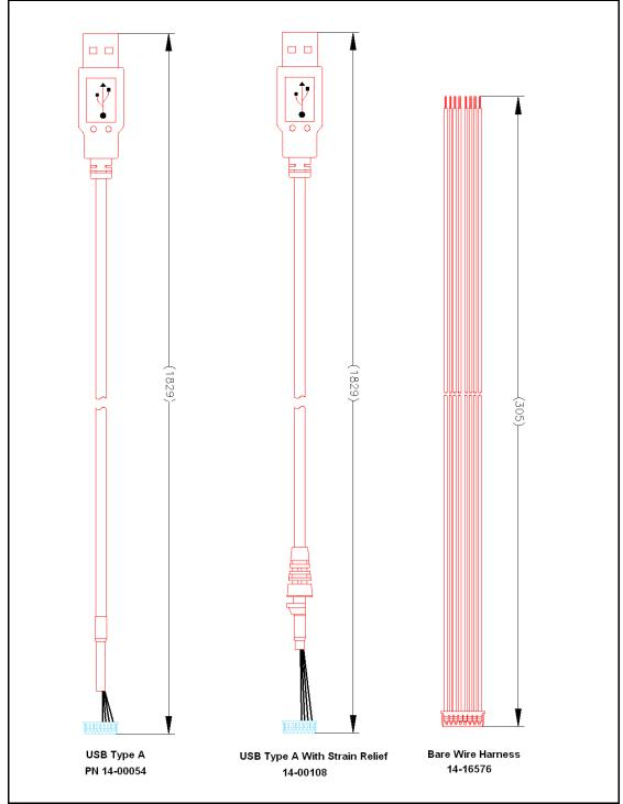
Figure 11: USB VersaPad Standard Cable Options
