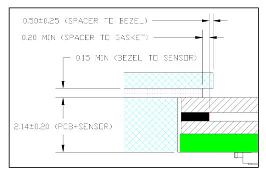
Figure 5: Critical capture dimensions. Drawing is not to scale.
