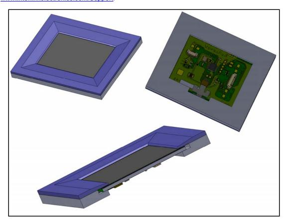
Figure 3: VersaPad Module Bezel Mounting Concept
