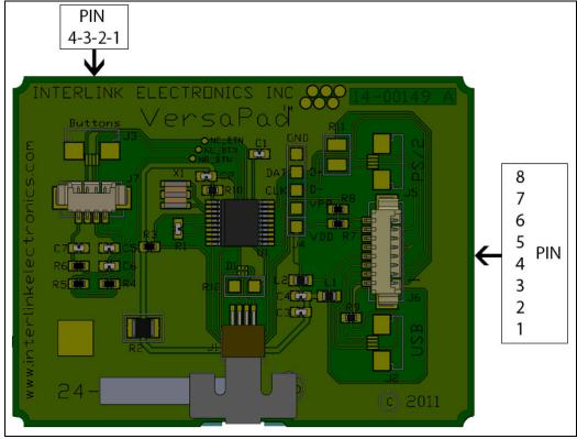
Figure 9: Molex Header Pin-Outs
