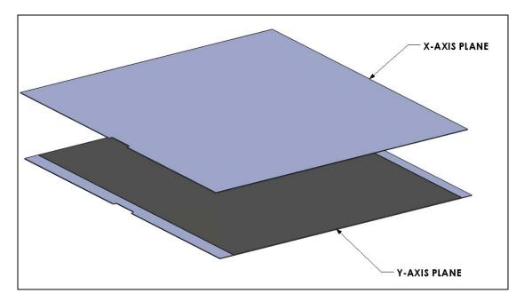
Figure 2: Simplified Exploded View VersaPad Sensor
