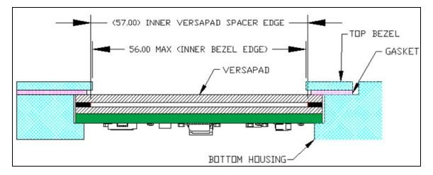
Figure 7: Side view of top side mounting. Drawing is not to scale
