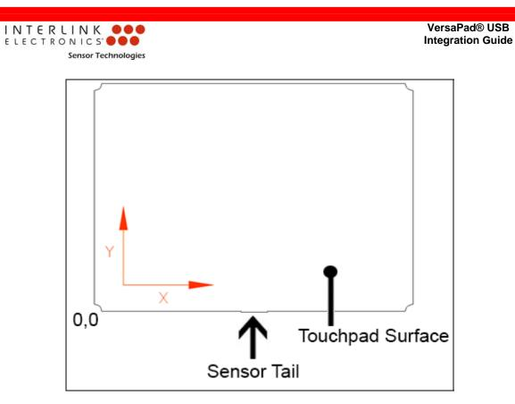
Figure 13: VersaPad default orientation
