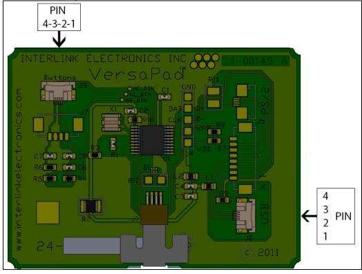
Figure 10: FFC Connector Pin-Outs
