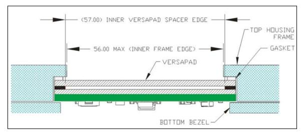
Figure 6: Side view of bottom side mounting. Drawing is not to scale
