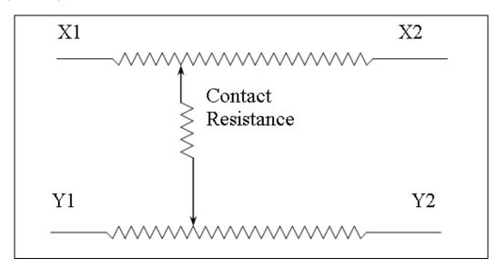
Figure 1: VersaPad Equivalent Electrical Circuit
