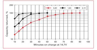
Table 7 shows that with a 0.8C10 inrush current, a 100% discharged battery can have 80% of its capacity returned in 57 minutes; doubling the inrush to 1.6C10 cuts the time taken to reach 80% capacity to only 28 minutes.
