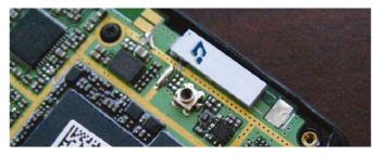
These highly innovative antennas provide competitive advantages for designers of cell phones, laptops and other mobile equipment by combining GPS & Bluetooth antennas in a single, highly compact form factor suitable for the thinnest/smallest devices. Ethertronics Isolated Magnetic Dipole (IMD) technology utilizes superior RF isolation to deliver the utmost in high performance.
