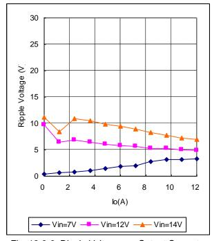
Fig. 12-3-6. Ripple Voltage v.s. Output Current
