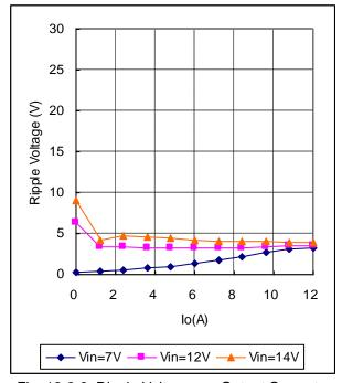
Fig. 12-3-3. Ripple Voltage v.s. Output Current
