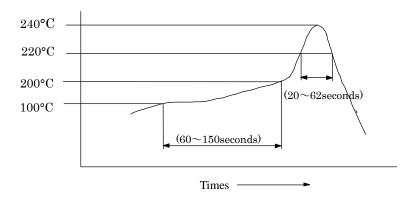
\*Do not vibrate for the products on reflow.
