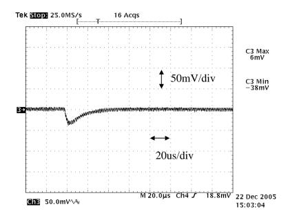
Fig. 12-1. Load Transient Response
